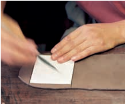
Paper stencils are used to cut out the necessary pieces used in the pot.
