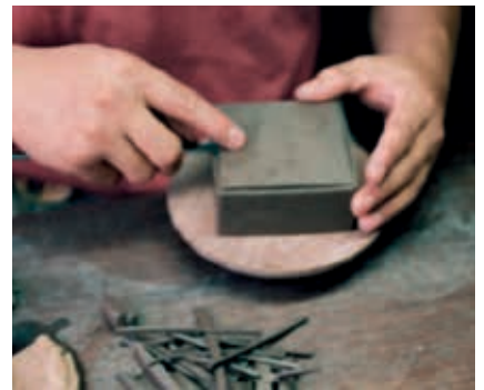
The top piece is then adhered to the body, forming a cube.
