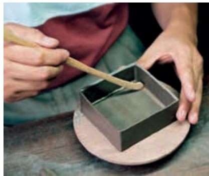
The creases of the joints are then smoothed out and refined.
