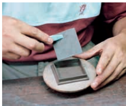
The lid and button are joined together and refined until they are smooth.
