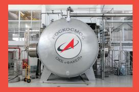
At Fakel's disposal, there are 20 vacuum chambers of 0.5 to 120 cubic meters in volume and up to 10<sup>-6</sup> Torr in pressure with cryogenic and other pumping systems. This state-of-art equipment allows to perform environmental test, thermal cycling test, mechanical test (i.e. sine vibration test, random vibration and shock tests), thermal vacuum and firing tests.
