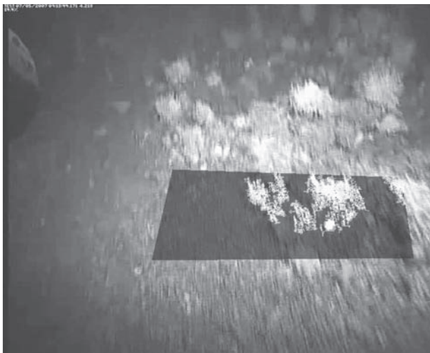
Figure 12 Candidate regions of stony coral detected using a colour signature. (Courtesy of CSIRO and SeaGIS Pty Ltd.)
