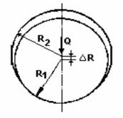
Fig. 1. The contact between a cylinder and a cylinder cavity
