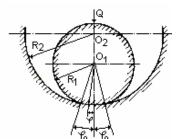
Fig.5. Contact between a cylinder and a cylinder cavity
