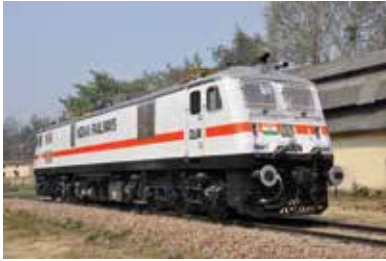
DLW Built first Electric Locomotive-6000 HP WAP7 Varun
