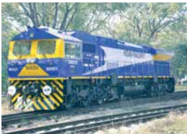
5500 HHP WDG-5 Diesel Electric main line heavy goods service locomotive
