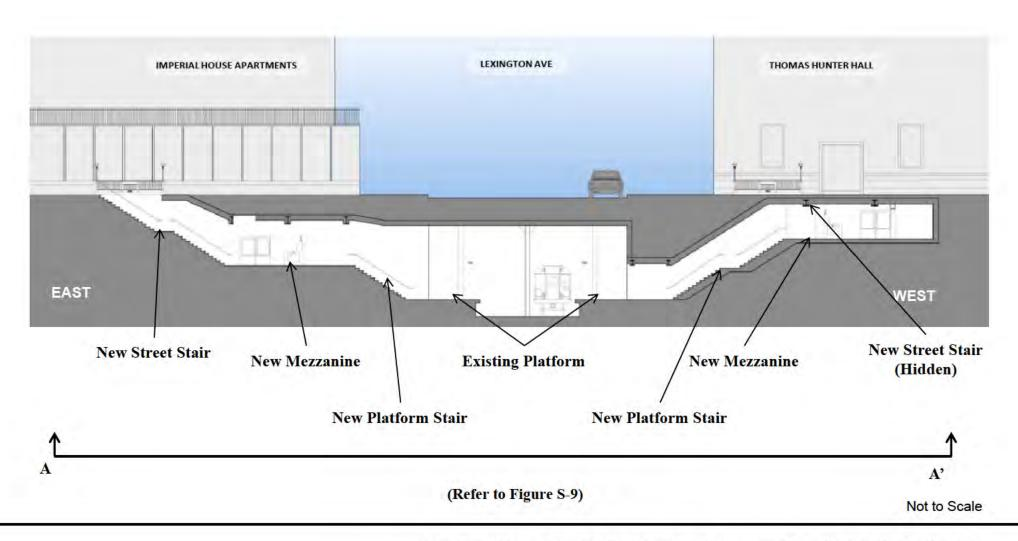
Section Along East 69<sup>th</sup> Street – Proposed Project with Option E1 Figure S-10
