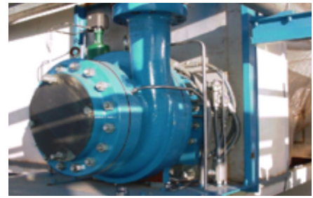
Air Products cryogenic expander typically used in the production of a small LNG plant.
