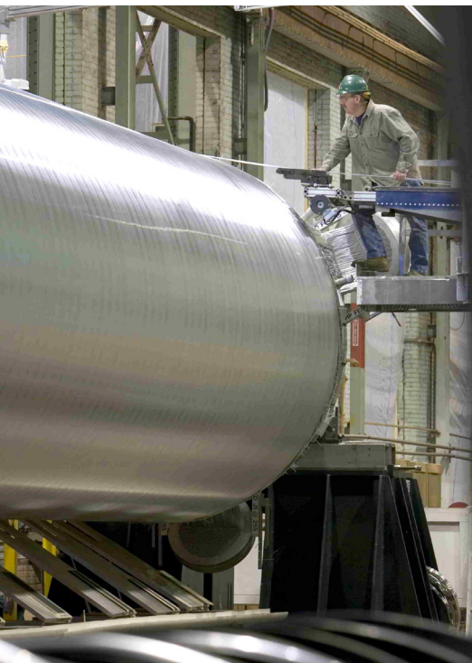
LNG heat exchanger bundle winding process.
