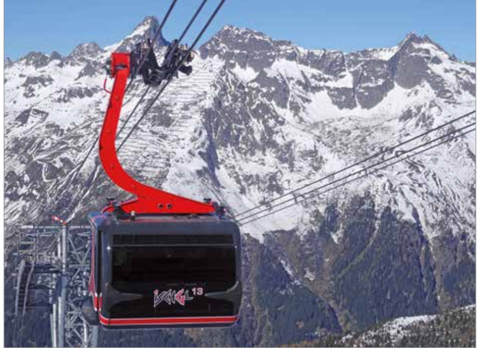
31 gondola cabins custom-designed by CWA for Ischgl take 28 passengers each to the ski slopes.
