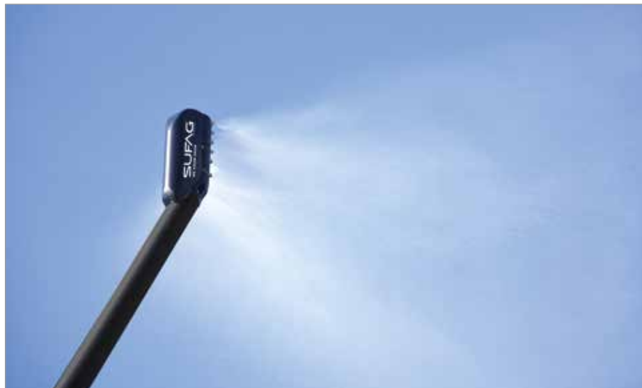
The new lance Taurus 2.0 starts at a wet-bulb temperature of -2^{\circ}\text{C} ( 28^{\circ}\text{F} ) and achieves a snow production of up to 25\text{ m}^3/\text{h} ( 880\text{ ft}^3/\text{h} ) at 60 bars (870 psi) water pressure. Photos: SUFAG
