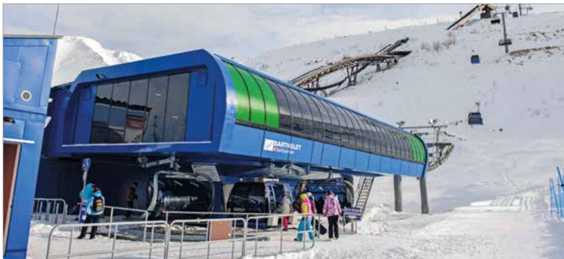
The combination line with offers a transport capacity to 2,400 P/h; trip time is 5.5 minutes at a speed of 5m/sec.
