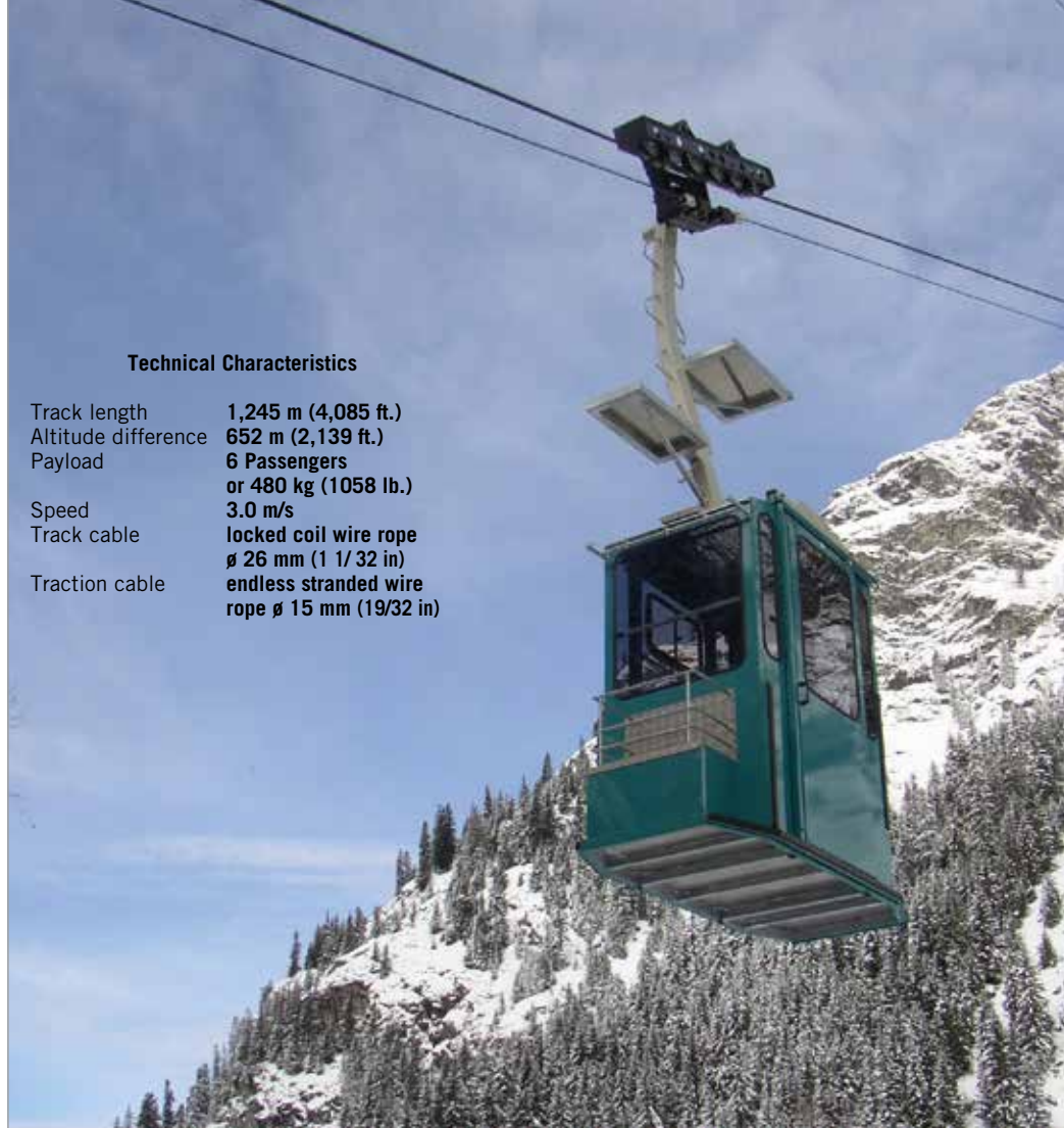
VON ROTZ & WIEDEMAR AG: a new vehicle, compliant with the EU cableways guideline 2000/9/EG.
