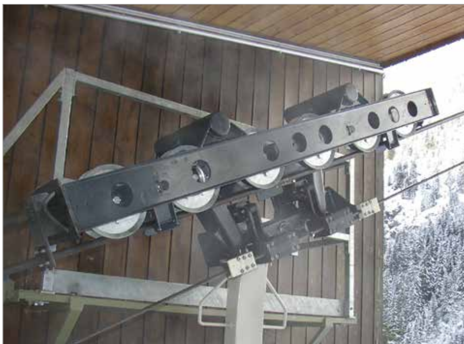
New carriage with clamps, without track rope brakes
