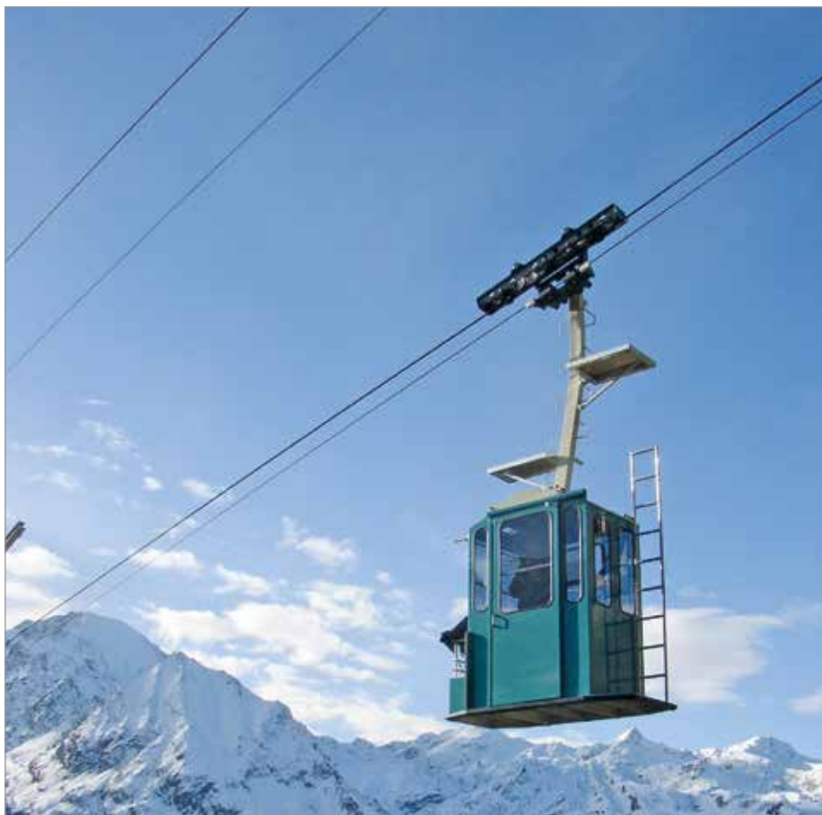
The cabin has an Aluminum-clad hot galvanized tubular steel frame.
