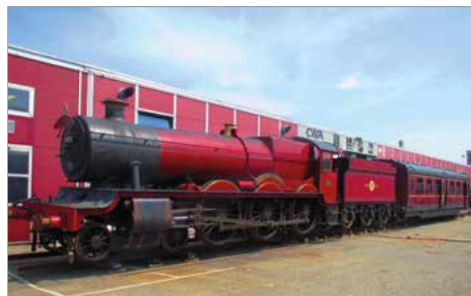
A train awaiting transport: The finished masterpiece outside the CWA production halls in Olten, Switzerland, weighs 100 tons, much less than its prototype. Visually, though, they are identical.
