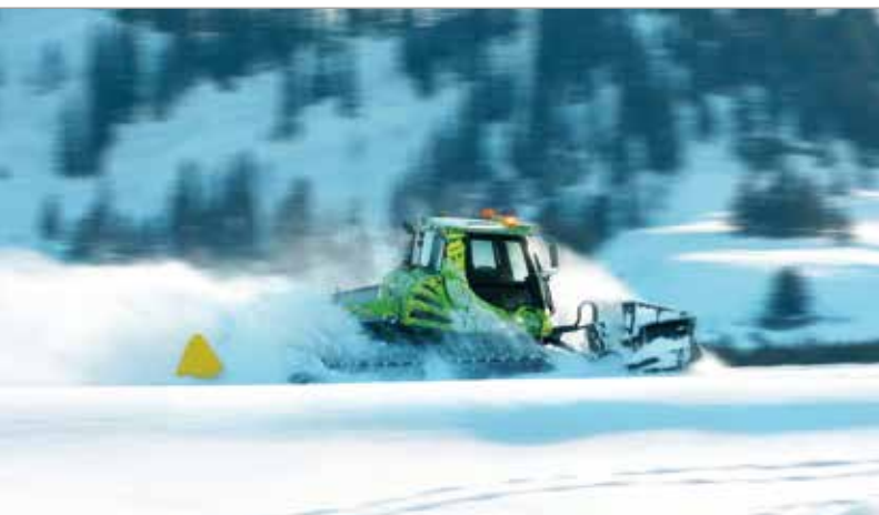
The PistenBully 600 E+ is the first snow groomer worldwide with a diesel-electric drive and is now also a genuine success story.
