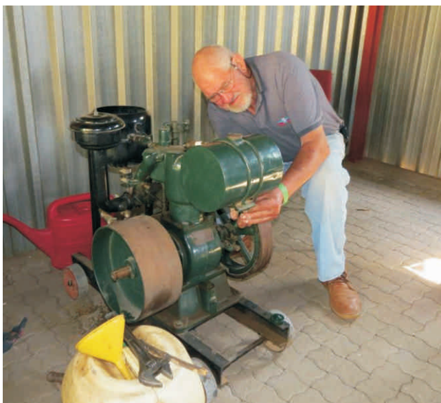
Dirk Brits cleaning the Massey Harris C34 (5HP) Fuel system to give it a test run
