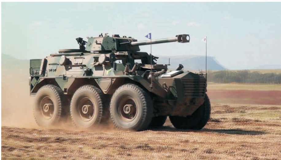
British designed but heavily South African modified Saracen Armoured Fighting vehicle with 90mm cannon at full stretch at Sandstone Estates
