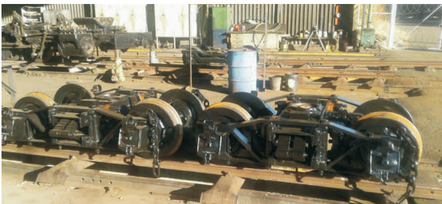
The remanufactured tender bogies with the refurbished main frames and motion in the background. Picture by Lukas Nel.
