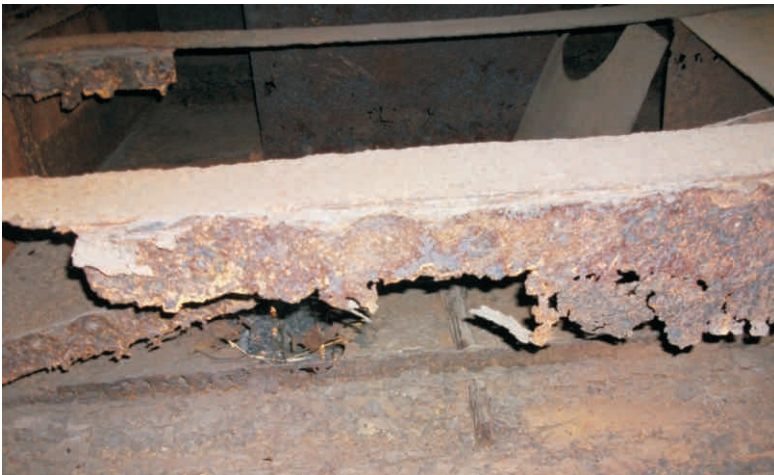
The new tender tank for the NG10 and below, an example of the wastage in the tender frames. Pictures by Lukas Nel.
