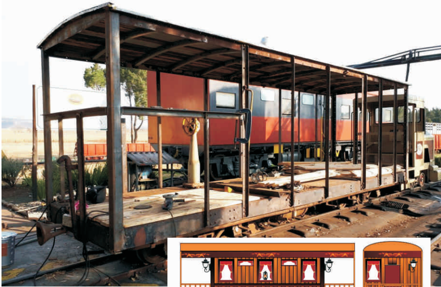
V16 Brake Van No 3170 begins its new life with conversion to a Lounge Car.
