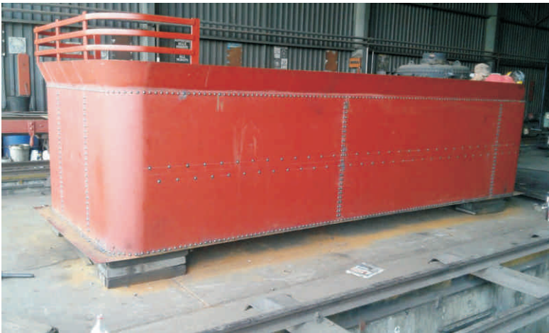
The new tender tank for the NG10 and below, an example of the wastage in the tender frames. Pictures by Lukas Nel.
