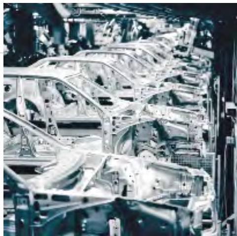
GUARANTEED RUST-FREE – FULLY GALVANISED BODY OF THE AUDI 80
