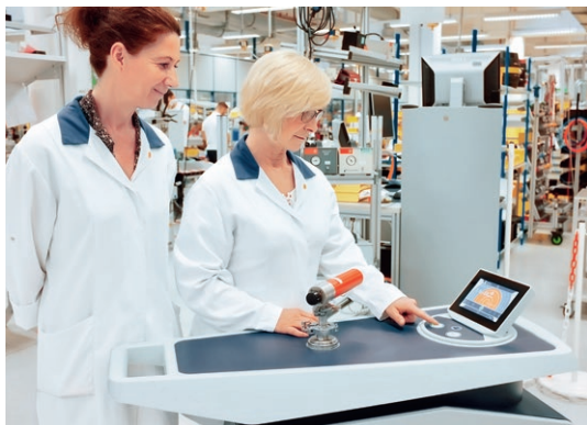
Leak detector UL3000 in use.
