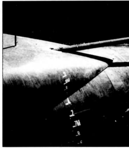
Before and after. Note the new more pointed after hull casing modification on HMAS COLLINS compared to HMAS WALLER (left). This is hoped to further reduce flow noise and cavitation around the propeller. (LAPH Erik Kennelly, RN & Rann Communications)
