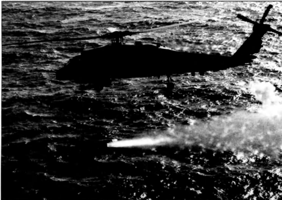
A USN SH-60 Seahawk fires a Penguin ASM. Seahawk is used by four regional countries, none of which use the Penguin except Australia but from its SH-2G Super Seasprites (USN).
