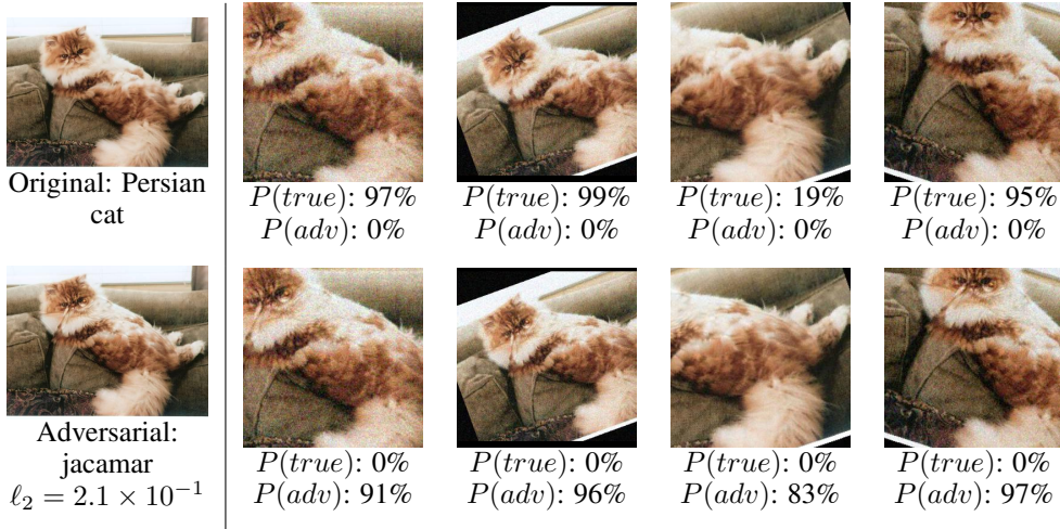
Figure 2: A 2D adversarial example, showing classifier confidence in true and adversarial classes for original and corresponding adversarial images over randomly sampled poses.
