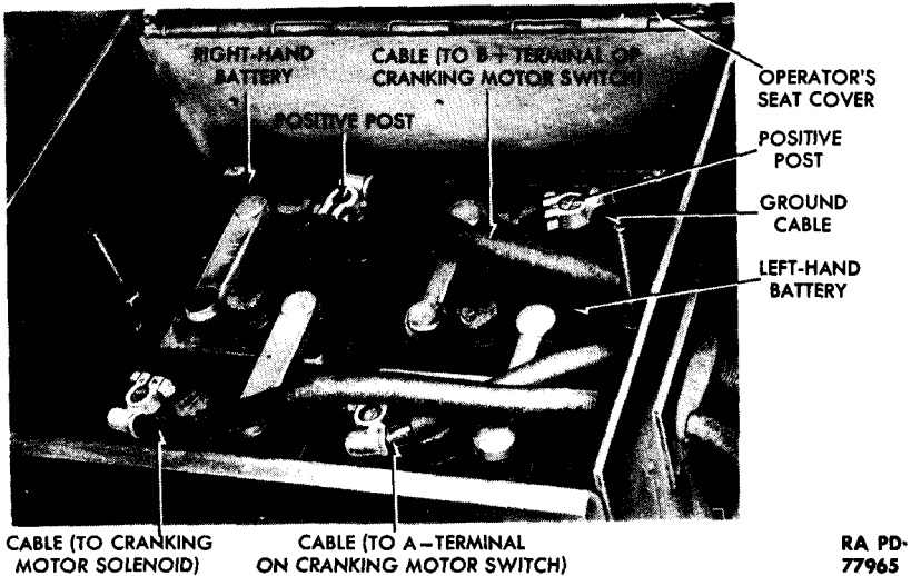
Figure 97 – Batteries Installed
