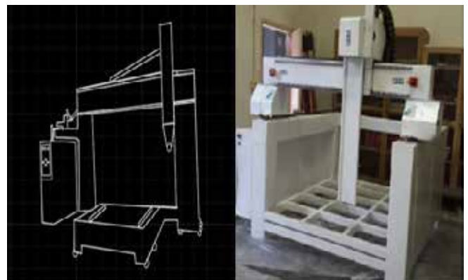
Figure 1. AutoCAD drawing of the machine and the actual manufactured CNC
