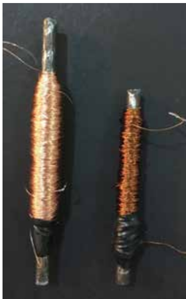
Figure 4: Two types of electromagnets fabricated- 0.1mm diameter to the left and 1mm diameter to the right
