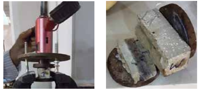
Figure 4. Bond test apparatus (left) and epoxy failure (right)
