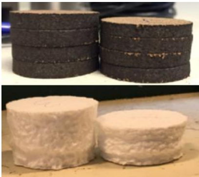
Figure 6. UTM specimens before (left) and after compression (right): MAC (top) and EPS(bottom)
