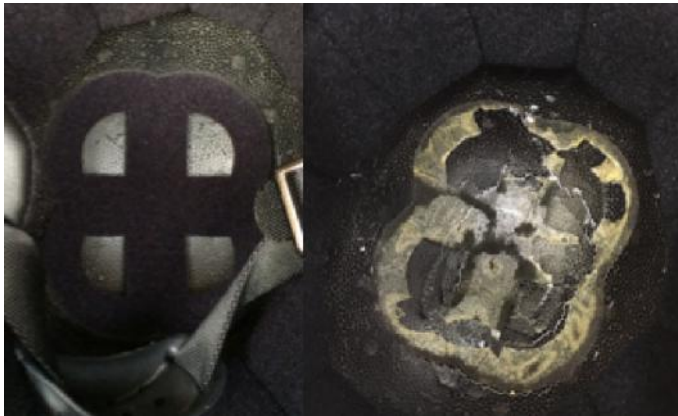
Figure 8. EPS liner crushed (right) at crown region after impact
