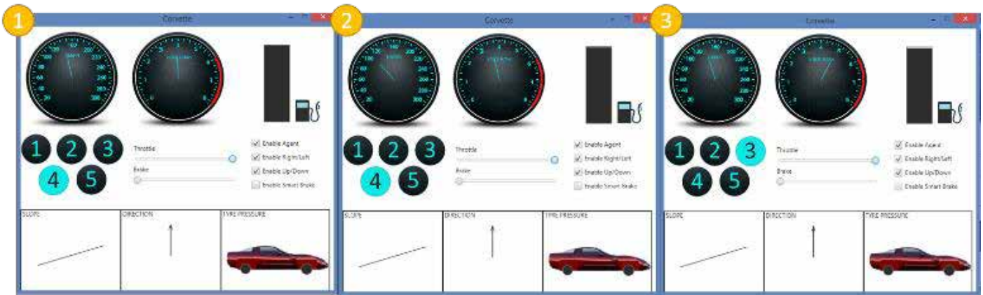
Figure 10: Test Case Number 4: From screenshot 1 to 2, one can notice the car decelerating despite full throttle being applied. In screenshot 3, the agent's response is shown. The agent lowers the gear allowing the car to regain acceleration.
