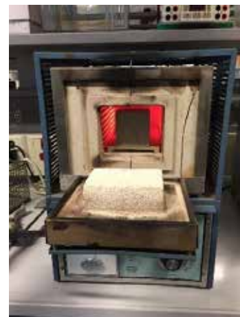
Figure 6. Concrete samples in the high temperature oven furnace.
