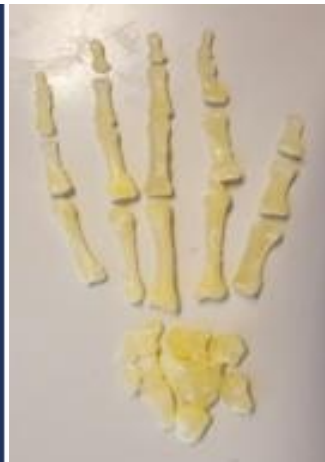
Figure 2: ABS printed bones
