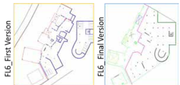
Figure 2: Transition of floor 6 to one coherent slab
