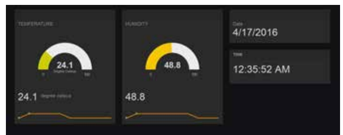
Figure 12: Dashboard showing data transmitted from the sensor to the cloud
