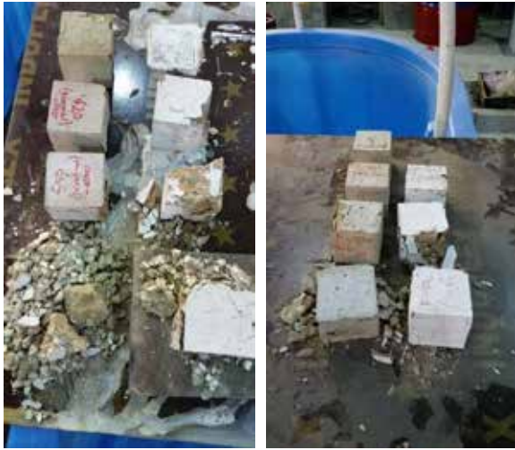
Figure 7. Plain concrete and fibers concrete samples after the compression strength test, from left to right.
