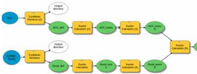
Figure 2. Model used to simulate noise propagation around AUBMC
