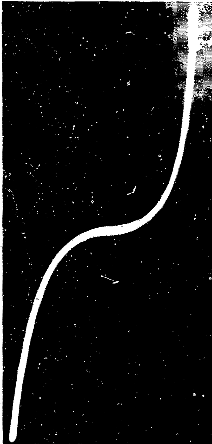
Figure 13. Oscilloscope image of I-V characteristic of Al/Al 2 O 3 /Mn/Pb diode driven by 60-cycle AC voltage at room temperature.
