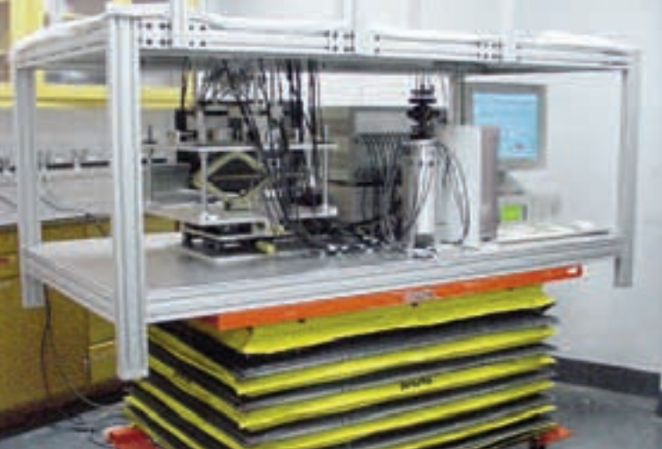
Left: Experimental imager setup for simultaneous dual breast optical mammography
