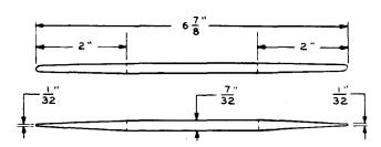
Primarily used in panel offices for testing commutator spring tensions. A wire position tool and other general use. **DO NOT USE FOR SOLDERING OPERATIONS.**
