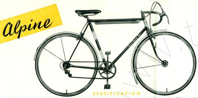
Frame: Built to angles 72°×71° with entirely new design of lug set with exclusive cutaway. Pump pegs under top tube. All brazed on fittings etc. Sizes 21°, 22°, 23°. EUUT tubing. Fork: Oval fork blades with special cutaway crown. Forged steel fork ends. Detachable lamp bracket. Wheels: 27″ Dunlop Endrick rims with Dunlop white side wall tyres. Large flange hubs. "S' motif on track nuts. Chainwheel: 46T 3/32°, 6½° cranks. "S' motif nuts on chainring. Fluted cranks. Brakes: New Sun "Wasp" alloy
