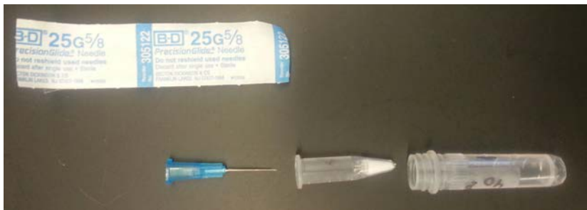
Figure 7-1. The needle is used to puncture the smaller 0.5 mL tube. The 0.5 mL tube is filled with a silica-containing compound. This is then placed inside a larger flat bottom 2.0 mL tube to form the DIY miniprep column.
