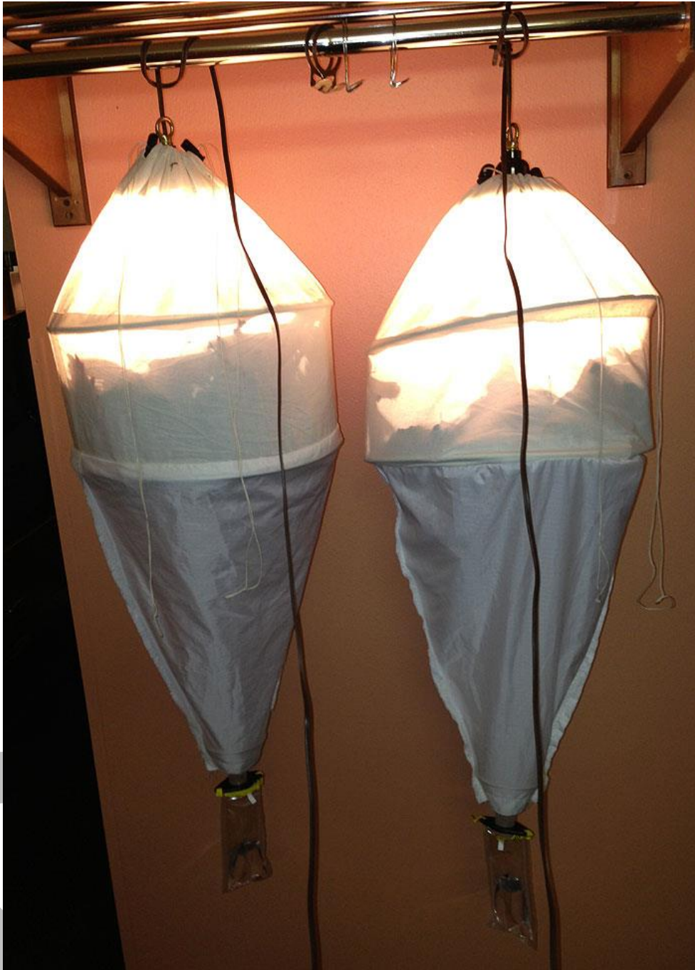
Figure 9. Collapsible Berlese funnels used to extract leaf litter fauna. The upper, cylindrical compartment is filled with leaf litter collected from the cave. Above it is suspended a 25 watt light bulb. The litter sits upon a coarse mesh (1/2 inch) hardware cloth, above a slippery cloth funnel, leading down to a container partially filled with ethanol preservative (and a sample label). Invertebrates in the litter move downwards in response to heat and drying, and are captured in the preservative. Photo by Steven J. Taylor.
