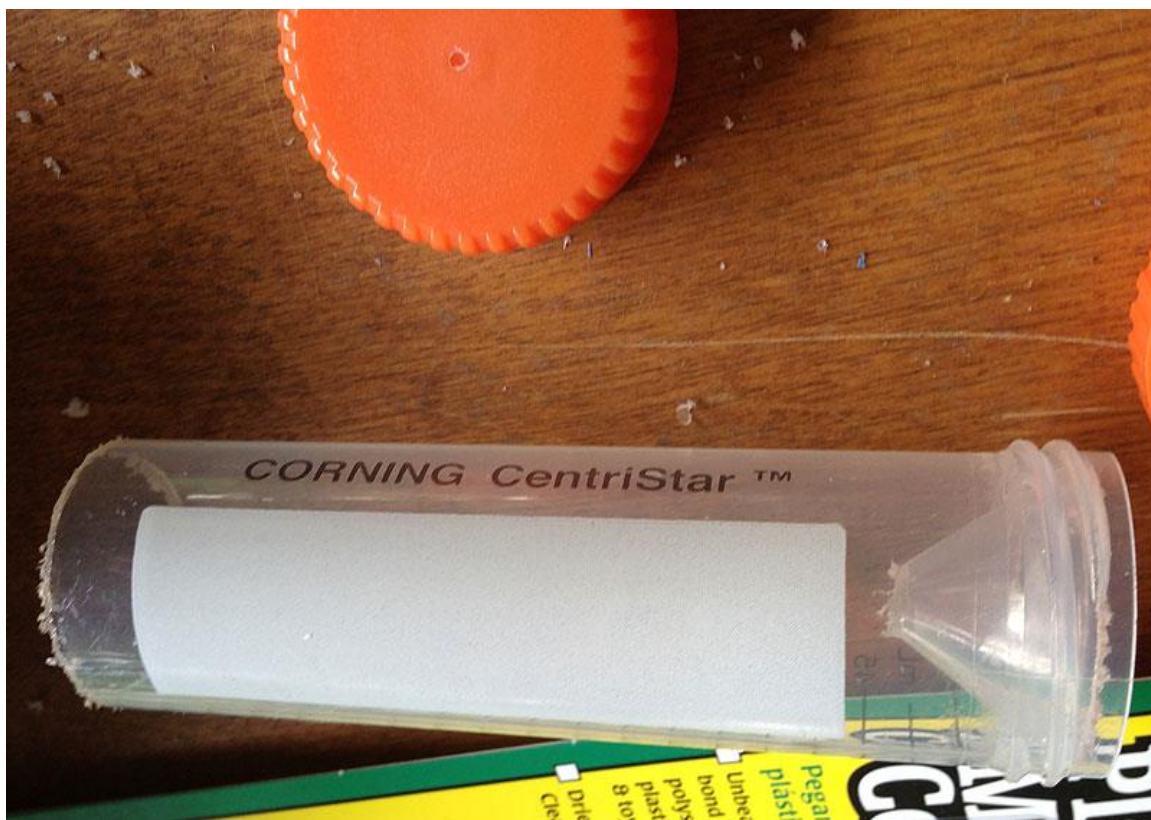
Figure 10. Nearly completed funnel trap constructed from a 50 ml centrifuge tube. Photo by Steven J. Taylor.
