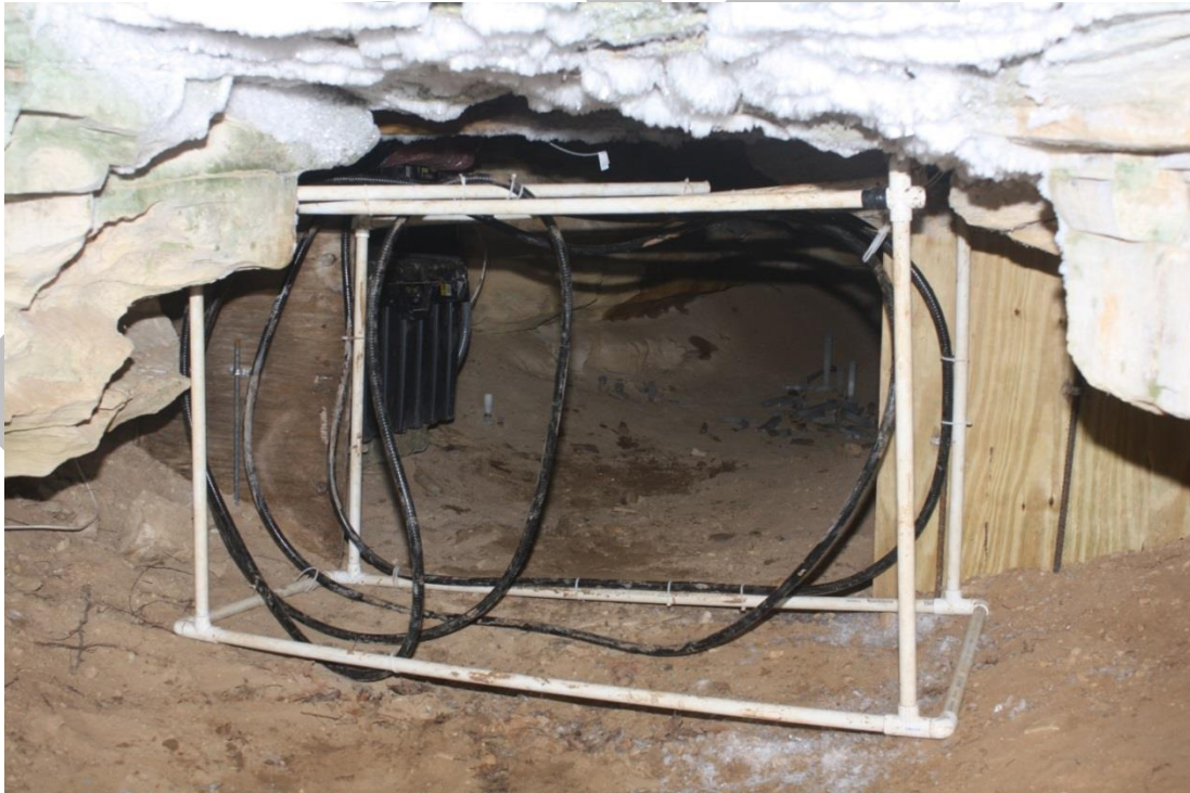
Figure 53 A looped PIT tag reading antenna was placed near the entrance to HSB Cave in 2014.
