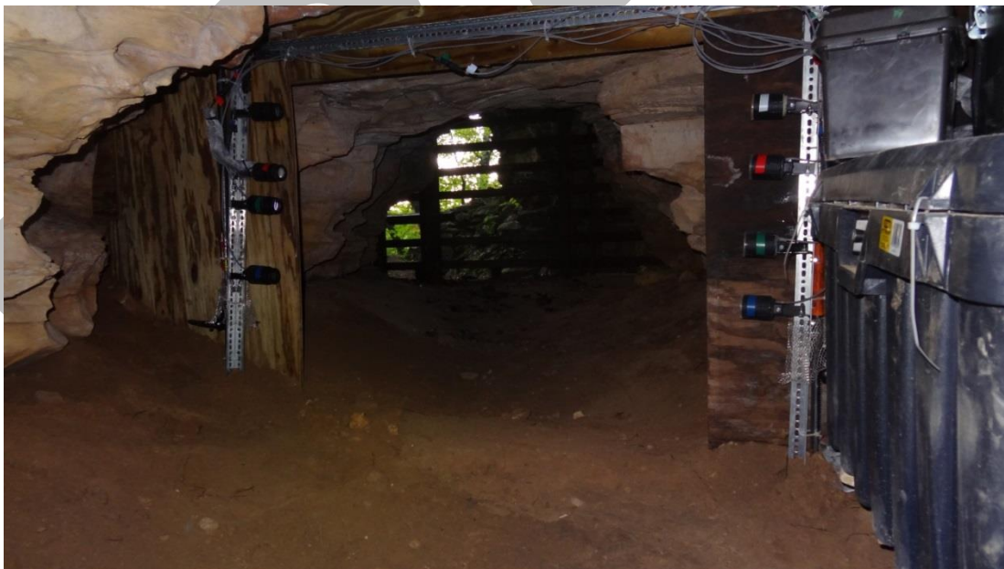
Figure 51 An infrared beam-break detection system was installed near the entrance of HSB Cave in the summer of 2013.
