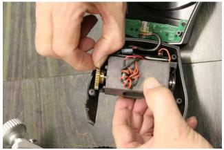
The gear that Mike is holding was extremely loose and this caused the sloppiness whenever the drive was engaged. Watch that you do not damage the encoder wheel on the right side. Tighten and reinstall by reversing the directions above.
