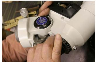
Remove the hex screw between the latitude adjusting screw and the polar scope.
