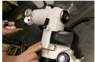
With the LXD75 in the counterweight down position (No counterweights, bar or scope) remove the 2 hex head screws on each side of the plastic housing.
