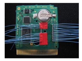
Cover all pin's (except pin 5, 6, 7, 8) with a piece of tape and solder the AM29F032B-90SD with pin 7, 8, 9, 10 directly to these 4 pin's.
