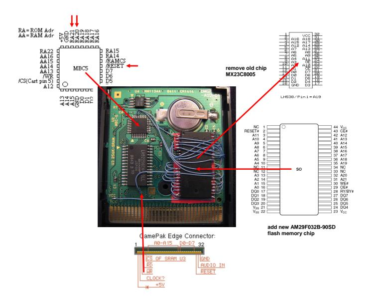
Connect the AM29F032B-90SD pin's to the corresponding pin's described inside the pin table for ROM chips and FLASH chips.
