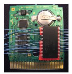
The tape is necessary to avoid any short between the PCB pin's and the flash chip.
