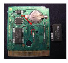
After that, solder 5 cm wires on each pin, except pin 5, 6, 7, 8.
