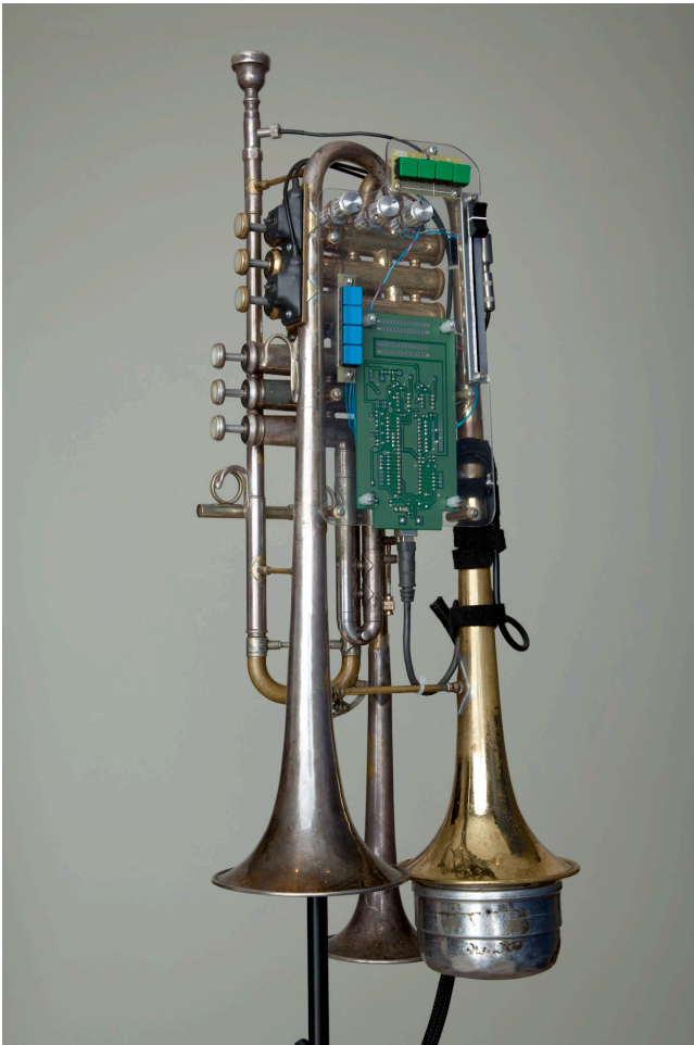
Figure 1. The current version of the mutantrumpet
