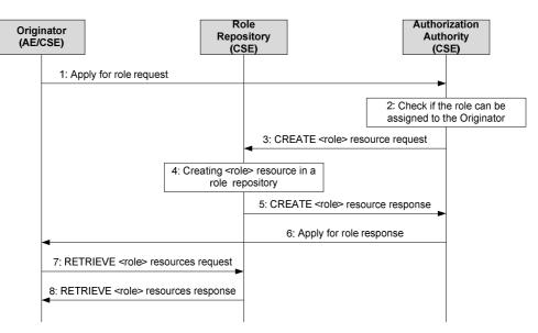
Figure 7.4.2.2-1: Procedure of role assignment
