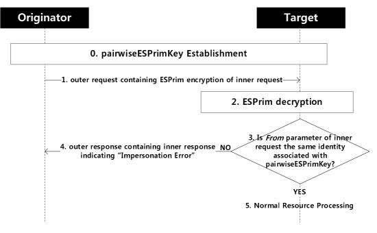
Figure 7.2.2-1: AE impersonation checking procedure
