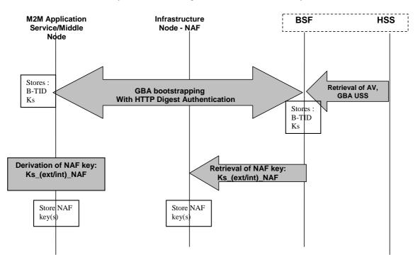
Figure 8.1.3-1: GBA framework. Note that the Network application Function (NAF) may be an Infrastructure Node or an M2M Authentication Function
