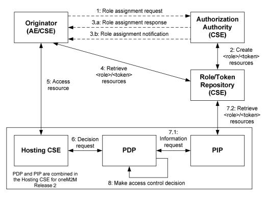
Figure 7.4.1-1. Role based access control architecture
