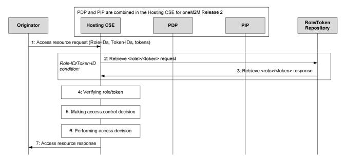
Figure 7.4.3-1: Role based access control procedure
