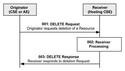
Figure 10.1.4-1: Procedure for DELETING a Resource
