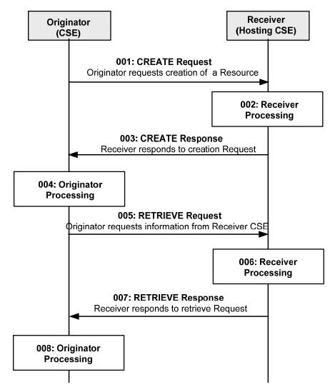
Figure 10.1.1.2.1-1: Procedure for CREATEing a <remoteCSE> Resource
