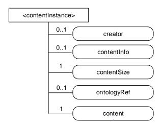
Figure 9.6.7-1: Structure of <contentInstance> resource
