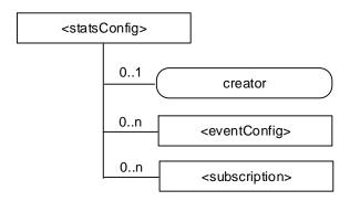
Figure 9.6.23-1: Structure of <statsConfig> resource
