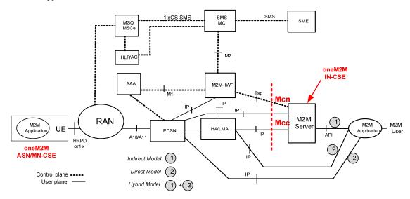
Figure C.3-1: Enhanced 3GPP2 Network Architecture for Supporting M2M
