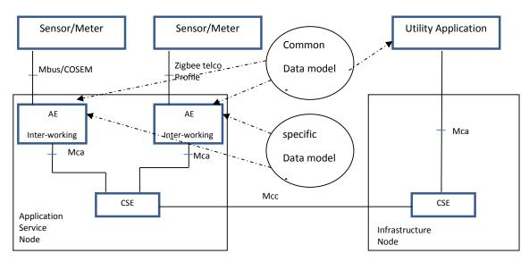
Figure F.2-3: Translation of non-oneM2M Data Model to oneM2M Specific Data Model
