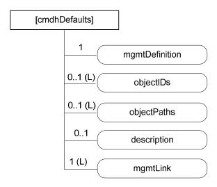
Figure D.12.2-1: Structure of [cmdhDefaults] resource
