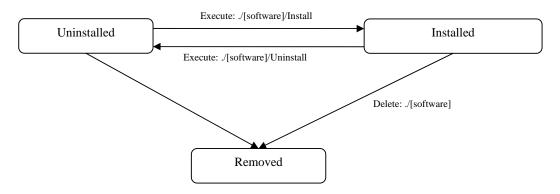
Figure D.3-2: State machine for [software] management
