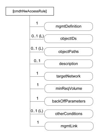
Figure D.12.7-1: Structure of [cmdhNwAccessRule] resource
