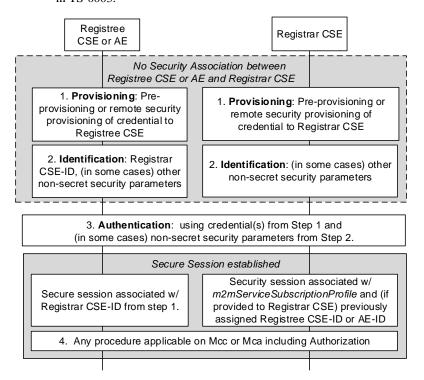
Figure 11.3-1: High Level Procedures on Mcc or Mca
