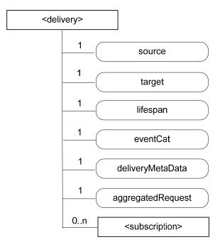
Figure 9.6.11-1: Structure of <delivery> resource
