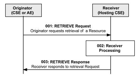
Figure 10.1.2-1: Procedure for RETRIEVing a Resource
