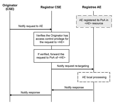
Figure 9.3.2.3-1: Re-targeting a notification request to an AE
