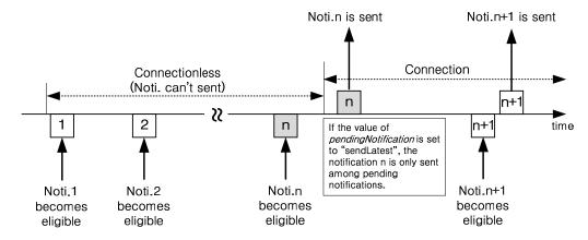
Figure 10.2.12-1: Notification Mechanism when pendingNotification (sendLatest) is used
