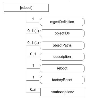
Figure D.10-1: Structure of [reboot] resource
