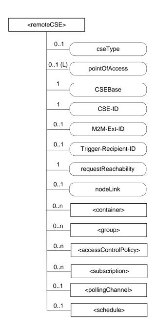
Figure 9.6.4-1: Structure of <remoteCSE> resource
