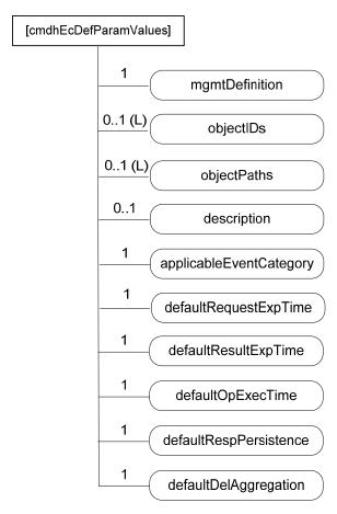
Figure D.12.4-1: Structure of [cmdhEcDefParamValues] resource
