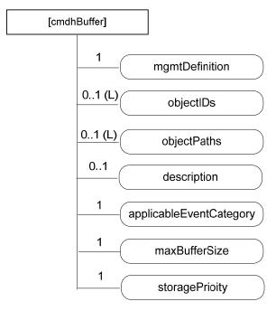
Figure D.12.8-1: Structure of [cmdhBuffer] resource
