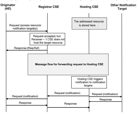
Figure 8.2.2.3-1: Non-blocking access to resource in asynchronous mode (Hosting CSE not equal to Receiver - 1 CSE), Originator provided targets for notification
