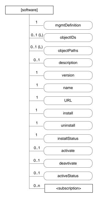
Figure D.3-1: Structure of [software] resource
