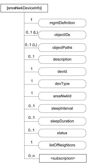
Figure D.6-1: Structure of [areaNwkDeviceInfo] resource
