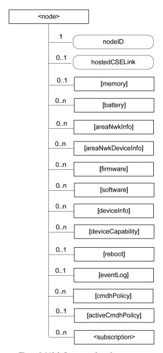
Figure 9.6.18-2: Structure of <node> resource
