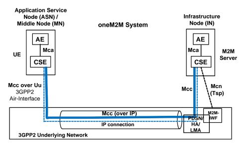
Figure C.4-1: User Plane and Control Plane Communication Paths
