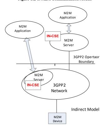
Figure C.2-2: Multiple M2M Applications Using Diverse Communication Models
