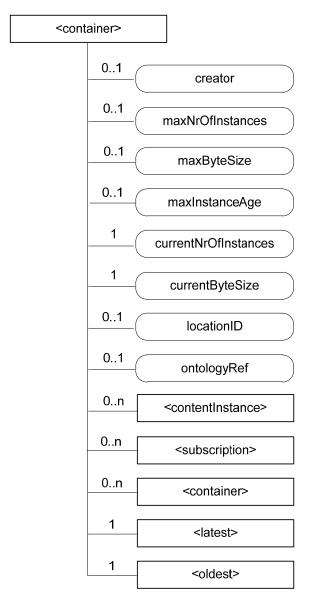
Figure 9.6.6-1: Structure of <container> resource
