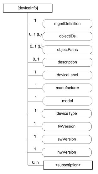
Figure D.8-1: Structure of [deviceInfo] resource
