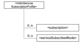
Figure 9.6.19-1: Structure of <m2mServiceSubscriptionProfile> resource
