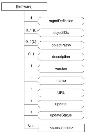
Figure D.2-1: Structure of [firmware] resource
