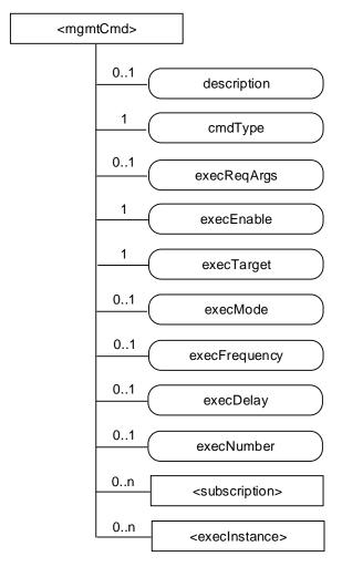
Figure 9.6.16-1: Structure of <mgmtCmd> resource
