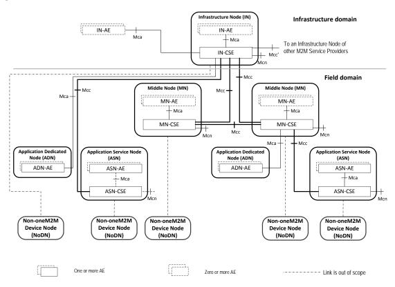
Figure 6.1-1: Configurations supported by oneM2M Architecture
