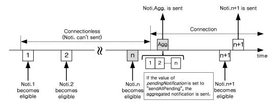
Figure 10.2.12-2: Notification Mechanism when pendingNotification (sendAllPending) is used
