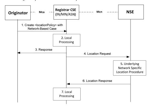
Figure 8.5.2-1: General Procedure for Location Request
