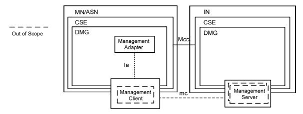
Figure 6.2.4.1.3.1-1: Management Client Interaction using "Ia" interface
