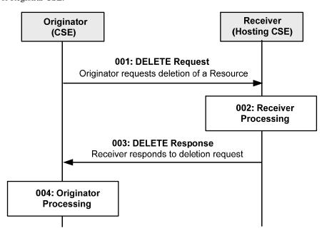
Figure 10.1.4.2.1-1: Procedure for DELETING a <remoteCSE> Resource
