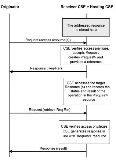
Figure 8.2.2.2-1: Non-blocking access to resource in synchronous mode (Hosting CSE = Receiver CSE), requested operation completed before second request
