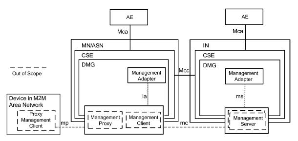
Figure 6.2.4.1.1-1: Device Management Architecture
