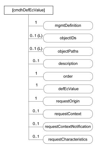
Figure D.12.3-1: Structure of [cmdhDefEcValue] resource
