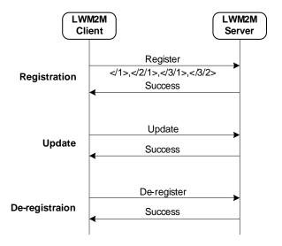
Figure A.5.3.2-1: Example of Registration Procedure
