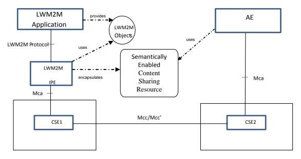
Figure 5.3-2: LWM2M Semantically Enabled Interworking Function
