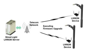
Figure A.1-1: Firmware Upgrade of Streetlight of Use Case using LWM2M
