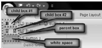
Figure 10-1: Nested box controls
