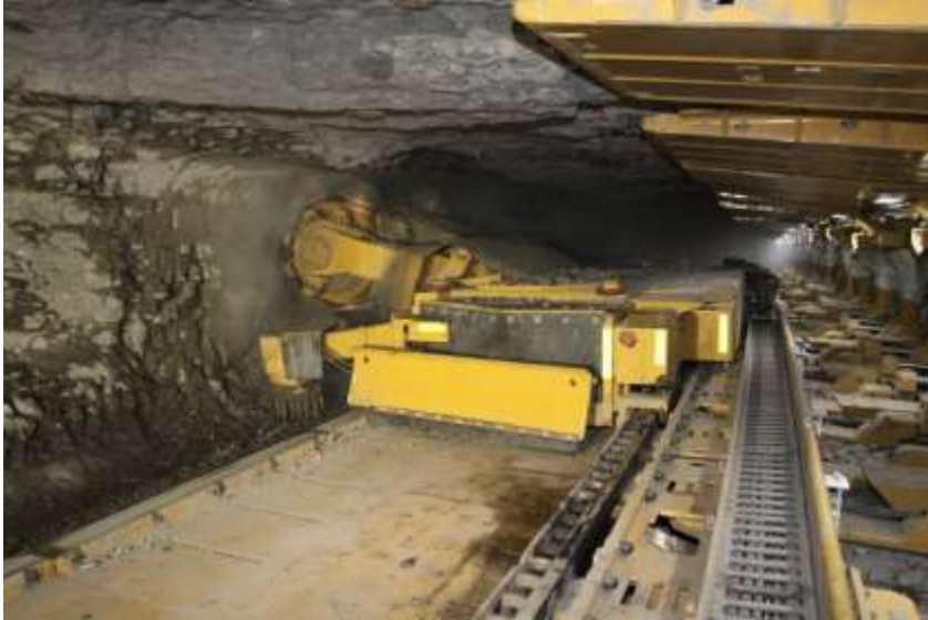
Testing the longwall complex (ACT Caterpillar, USA) with continuous mining at a copper ore mine, KGHM; 2014
