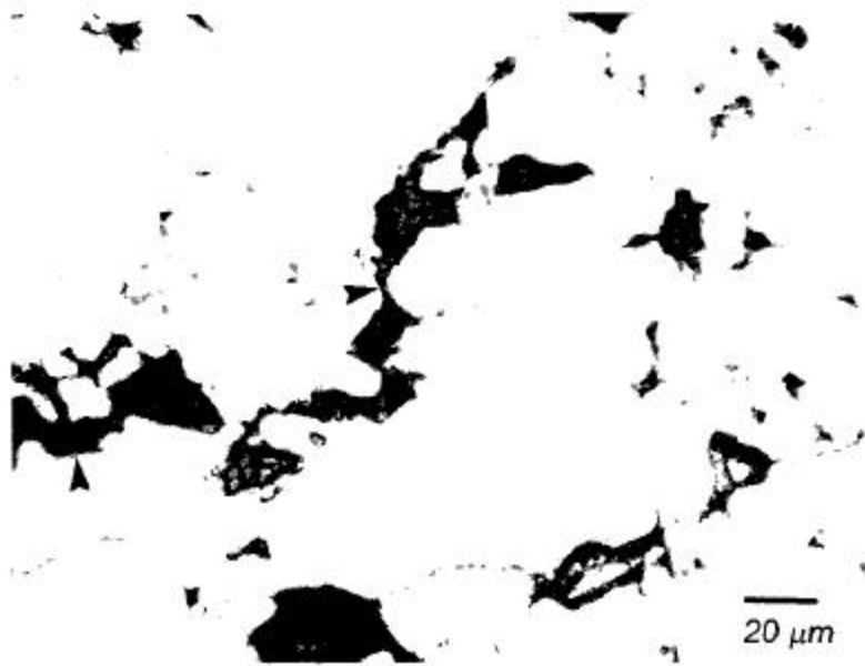
Figure 13: Microstructure of Green Compact for Material IB Showing Location of Zinc Stearate Between Particle Surfaces.
