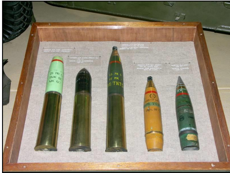
Figure 1 - Various 25 pr munitions – L to R: Smoke, Armour-piercing (Pre-1955 UK markings), HE (RDX/TNT), HE projectile (Amatol, Pre-1955 UK markings), Smoke projectile (Pre-1955 UK markings)
