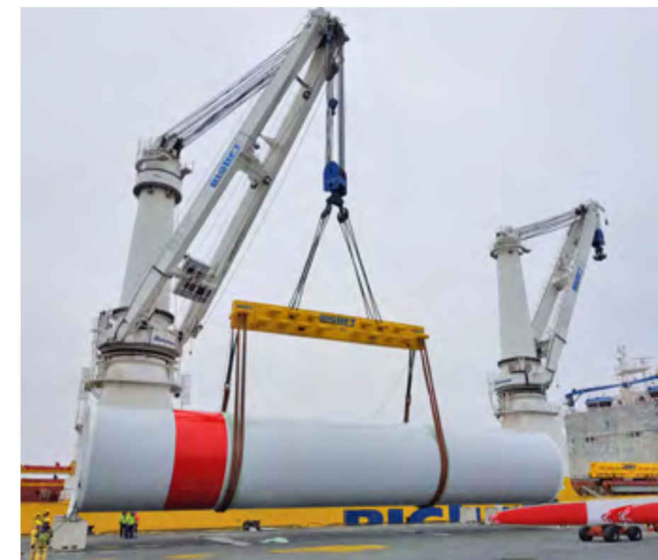
Happy Sky loading tower sections in Cuxhaven, Germany
