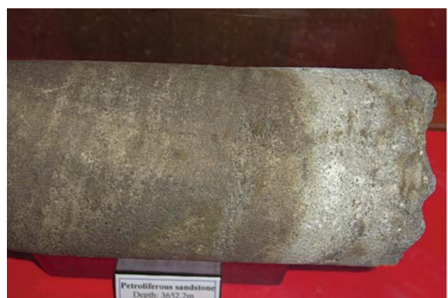
Fig.6. Non-uniform character of oil contamination of Oligocene reservoir - Bach Ho field
