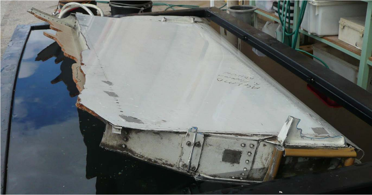
Fig. 2.1.3. Flaperon floating intrados up, viewed from inboard (no photo of 9M-MRO's is available).
