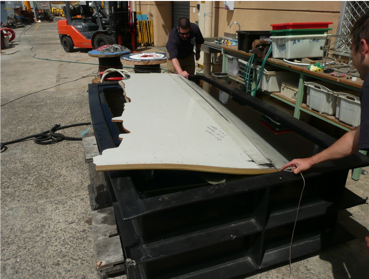
Fig. 2.1.2. Flaperons floating extradors up, viewed from outboard. The string shows the waterline.
