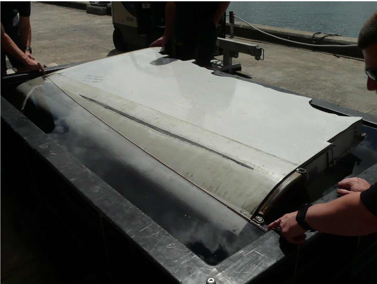
Fig. 2.1.4. Flaperon floating extrados up, viewed from inboard (no photo of 9M-MRO's is available). The string shows the waterline.
