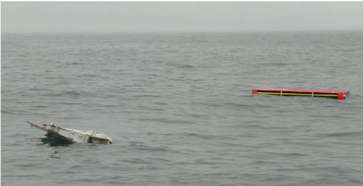
Fig. 1.1 The genuine and replica flaperons at sea in calm weather, having just been deployed (in an intrados-up orientation).
