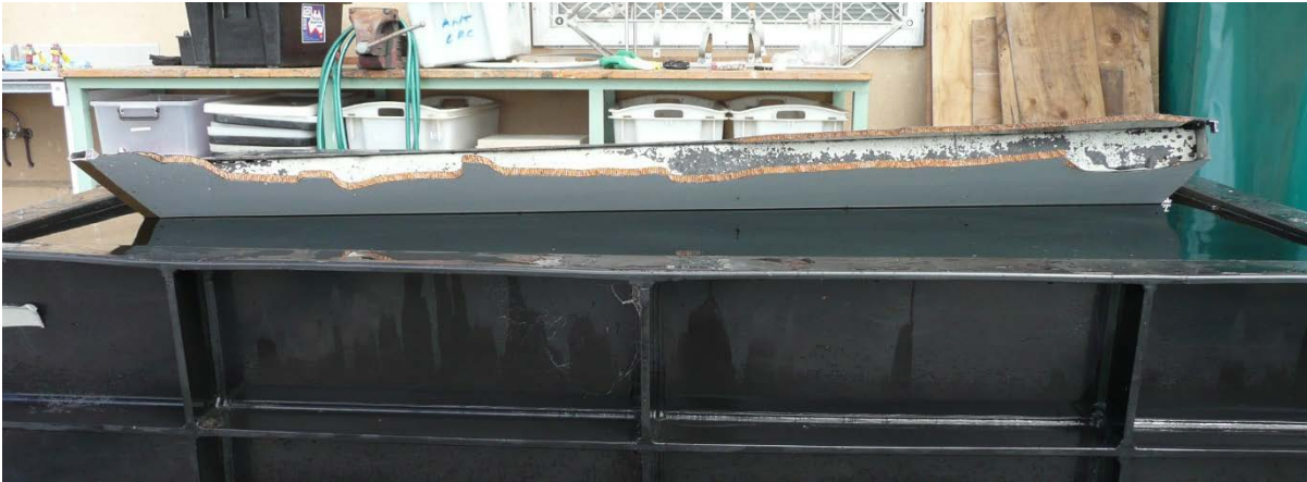
Fig. 2.1.5. Flaperon floating intrados up, viewed from the trailing edge (no photo of 9M-MRO's is available).
