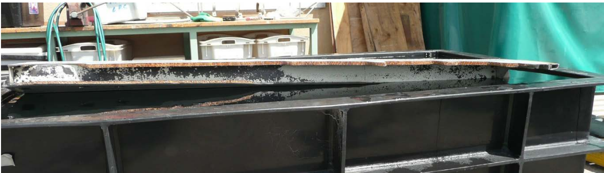
Fig. 2.1.6. Flaperon floating extrados up, viewed from the trailing edge (no photo of 9M-MRO's is available).
