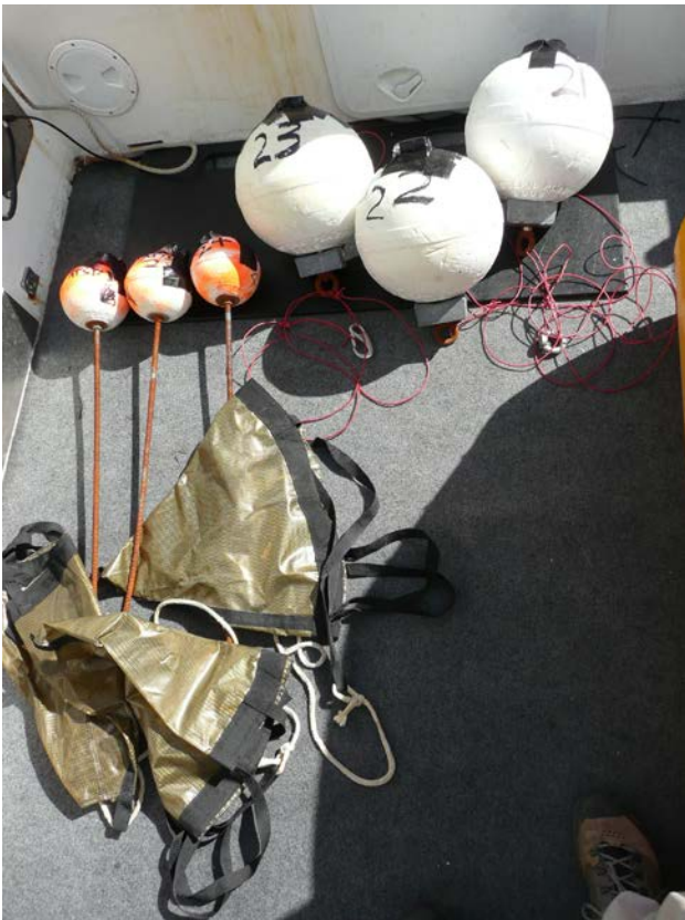
Fig. 2.2.2. Drogued (left) and undrogued (right) drifters, all fitted with GPS units taped on top. The 4kg of lead beneath the undrogued buoys puts the waterline equal to that of a similarly-sized GDP drifter once it has lost its drogue.
