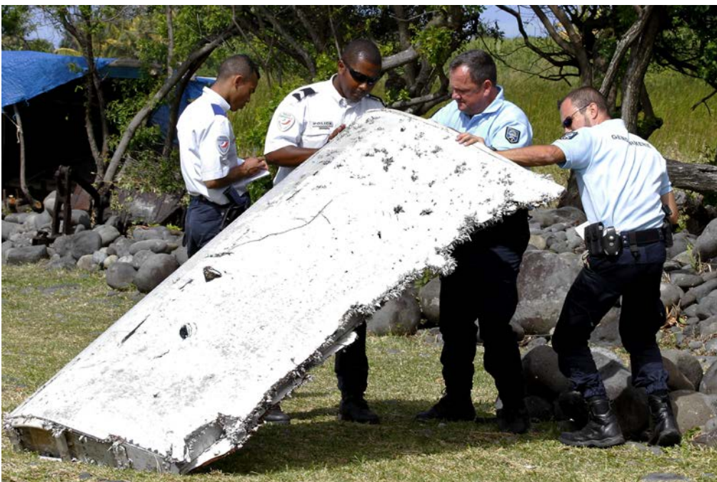
Fig. 2.1.7. Press photograph of 9M-MRO's right flaperon shortly after retrieval on Ile de la Reunion, showing a mild degree of barnacle encrustation on both the leading and trailing edges.
