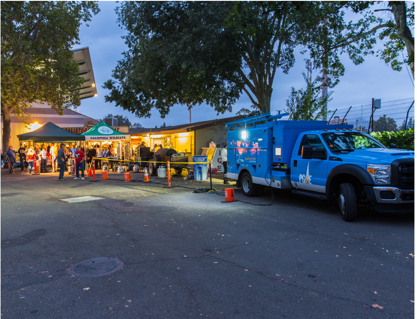
Pacific Gas and Electric work truck developed in partnership with Efficient Drivetrains, Inc (EDI) has the ability to export power for on-demand power when the grid isn't functioning. The above picture shows a PG&E truck powering a site at a Red Cross event in California.
