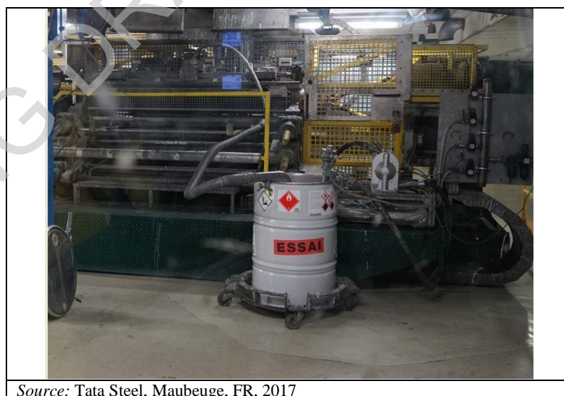
Figure 17.4: Paint supply at coating head in coil coating
