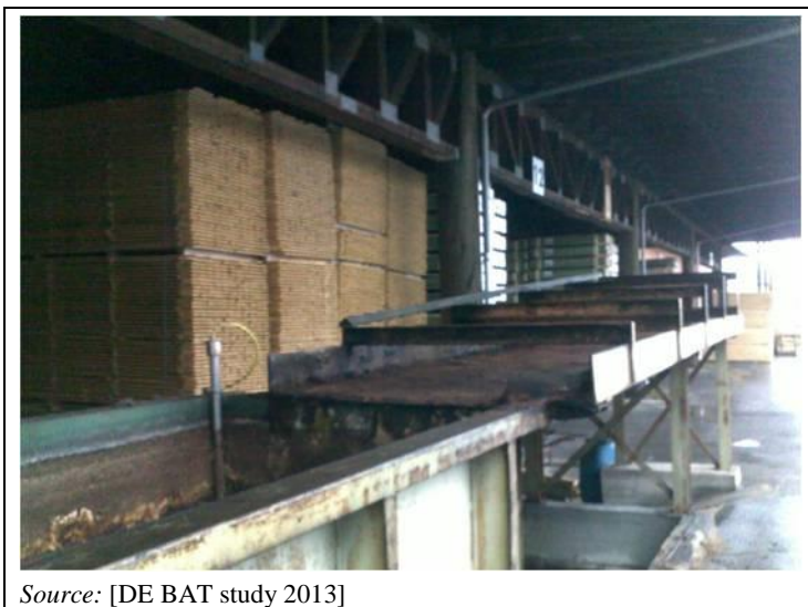
Figure 15.28: Example of a roof cover in the area of troughs (plant DE-4)
