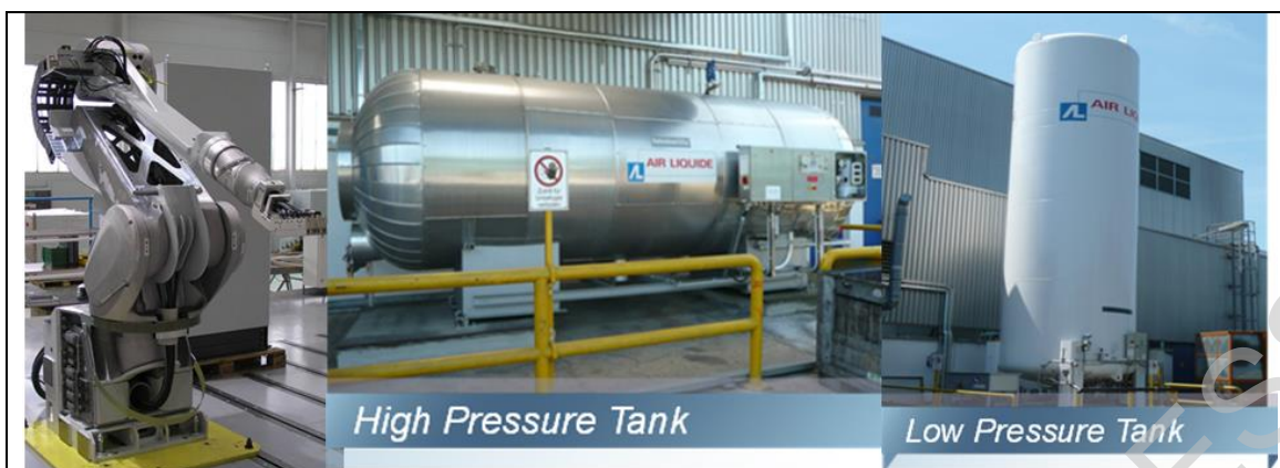
Figure 17.14:(a) Applicator robot (b) High pressure CO 2 tank (c) Low pressure CO 2 tank (Dürr)
