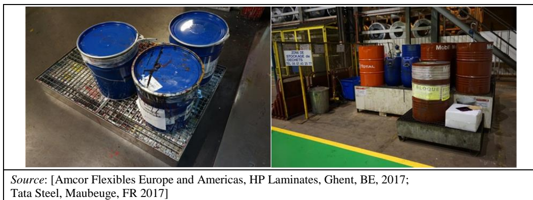
Figure 17.2: Built-in containment for moving and storing drums in production areas
