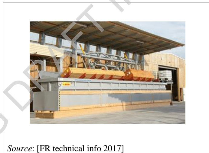
Figure 15.5: Example for brief dipping - tank allowing the simultaneous treatment of several batteries with the fixing done on racks next to the dipping tank
