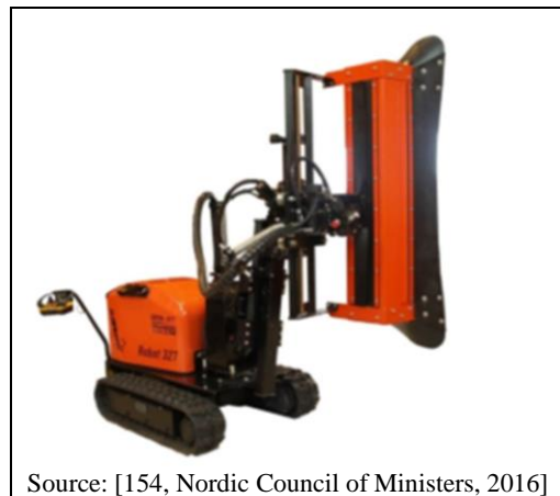
Figure 4.1: Box around the spear head in some more advanced robot models
