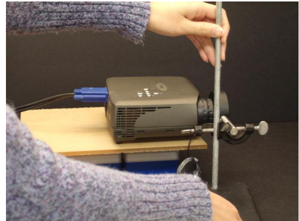
2. Put a magnifying glass (on a ring stand) in front of the projector, allowing light to pass through the lens.
