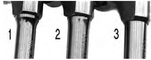
The three barrel profiles used with the Colt pre-Woodsman and First Series Target Model: from left to right, in order used, the pencil barrel, medium weight barrel, and straight taper barrel.
