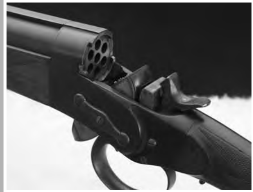
Closeup of the receiver of the Pieper Volley Gun. Note the general resemblance to the Remington Rolling Block
