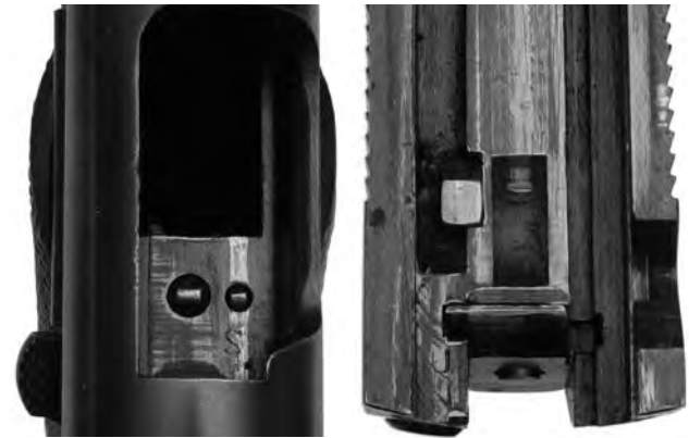
The Swartz pin is the smaller of the two pins, as seen from the top of the ejection port. The Swartz piston is located to the side of the disconnecter notch in the slide. Courtesy Karl Karash
