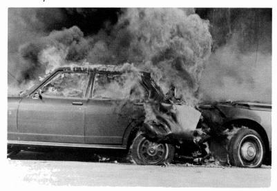
system rupture combines with a momentary spark from electrical components, crash friction, road flares or some other source." (See photo, upper right.)
