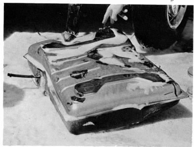
1973 Ford Galaxie 500 into a 1973 AMC Ambassador: "In this crash, the struck Ambassador's filler tube was allowed by the car's design to be torn from the hose that connects it to the fuel tank, and the tank itself was exposed to view . . . . A spark would have sent these cars up in flame literally in a split second. (See photo lower right.)
