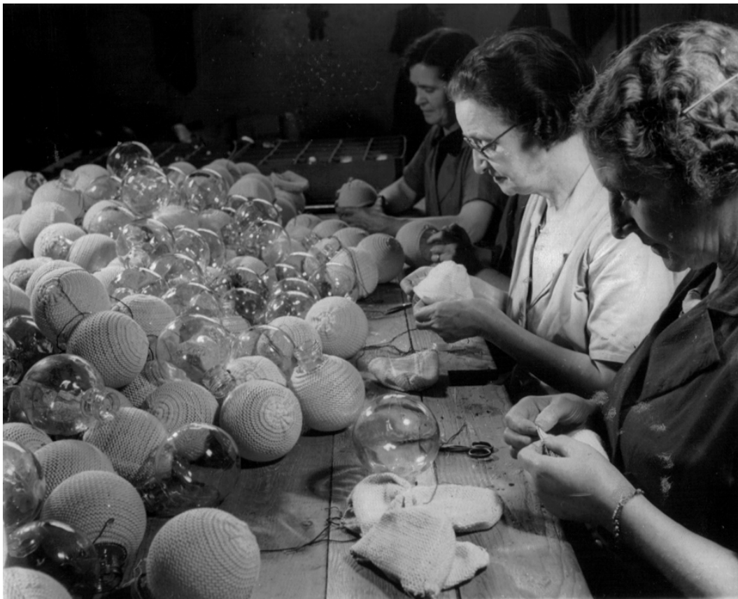
Released in July 1943, this official photograph is one of series showing the manufacture of ST grenades, 'just off the secret list', at Kay Brothers' Kayborough Works. Mrs Colman (nearest camera), Miss Brearley and their colleague are fitting 'woollen jackets' (which held the sticky glue) to each of the 2½ million grenades manufactured by the works. (Official photograph, author's collection)
