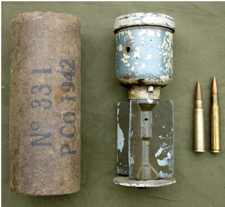
Practice No. 68 grenade (white painted body, centre) with its cardboard shipping tube (left) and a .303in and .300 rifle rounds for scale. (Author's photograph)
