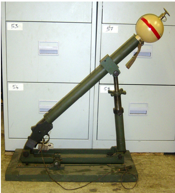
(Right) A mysterious 'take down' bomb thrower, with a barrel extension that stows in the base. The mount is also fitted with a plumb bob (inset below) to ensure that it is placed flat
