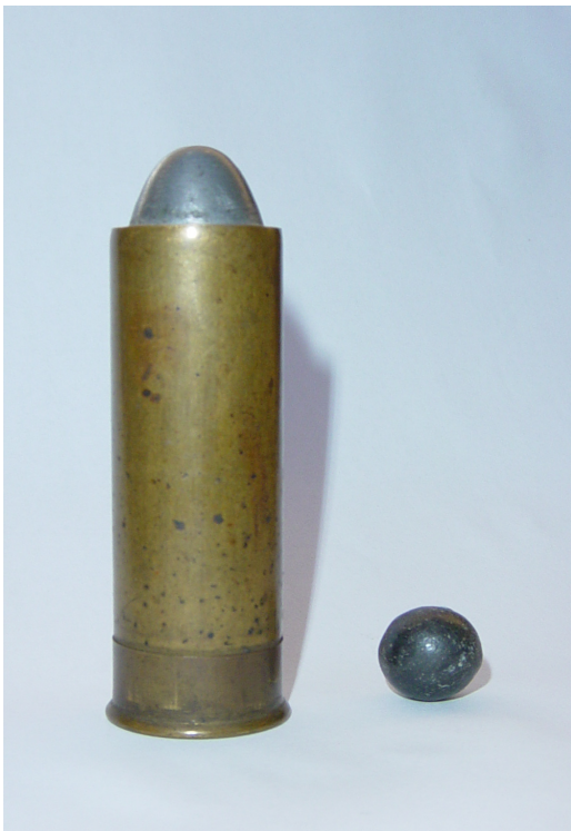
A 12-bore brass cased ‘Lethal Ball’ round by Kynoch (left) and half-inch shrapnel ball. (Author’s photograph)
