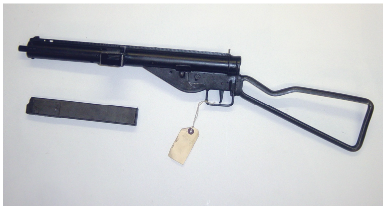
(Left) Sten Mk III. Produced from January 1942 by the makers of Tri-ang toys, the sheet metal and welded construction anticipated 'third generation' sub-machine guns. 876,886 were built at the company's Merton toy factory (Skenneron, 1988, p.34).
