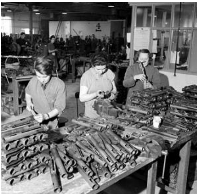
(Left) 1942, 'German and Hungarian women work on the manufacture of Sten guns at an ordnance factory, somewhere in Britain.' The photograph gives some impression of the volume and speed of Sten gun production by largely unskilled or semi-skilled workers. (IWM P869)
