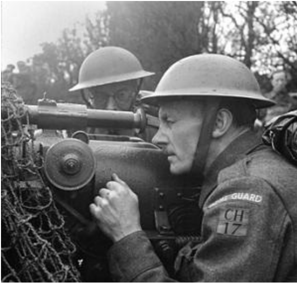
A hybrid 6pr anti-tank gun in service with the Home Guard – “Men of the Cheshire Home Guard man a 6 pounder naval gun mounted on a field gun chassis at Hoylake on the Wirral, 1 June 1943”. (IWM H30442)
