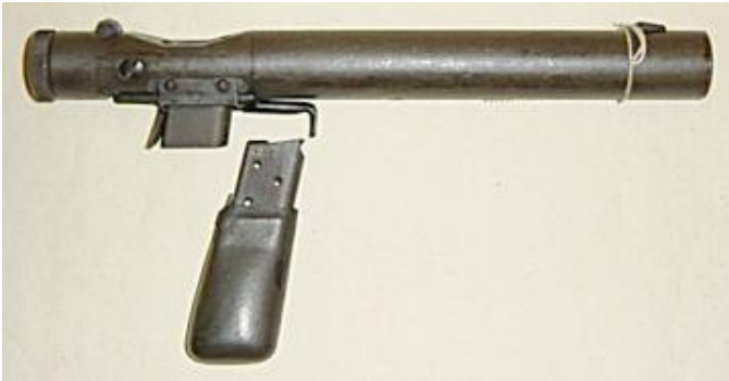
The .32in (7.65mm) Welrod Mk. II with magazine / pistol grip removed. (REME Museum)
