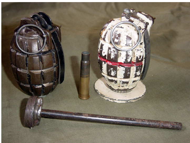
Mills bombs. No. 5 grenade dated 1916 (left), base plug and rifle discharging rod for a No. 23 grenade (front). A black stained (for identification) .303 Ballistite grenade launching blank (centre) and a No. 36M grenade of 1942 with gas check base plate fitted (right). This No. 36M is painted white for 'practice' with a red band for 'explosive filled', as it used an adapted detonator to give a puff of smoke for training purposes. (Author's photograph)
