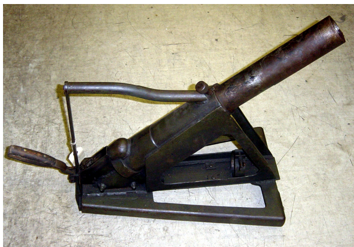
(Right) A mysterious 'take down' bomb thrower, with a barrel extension that stows in the base. The mount is also fitted with a plumb bob (inset below) to ensure that it is placed flat
