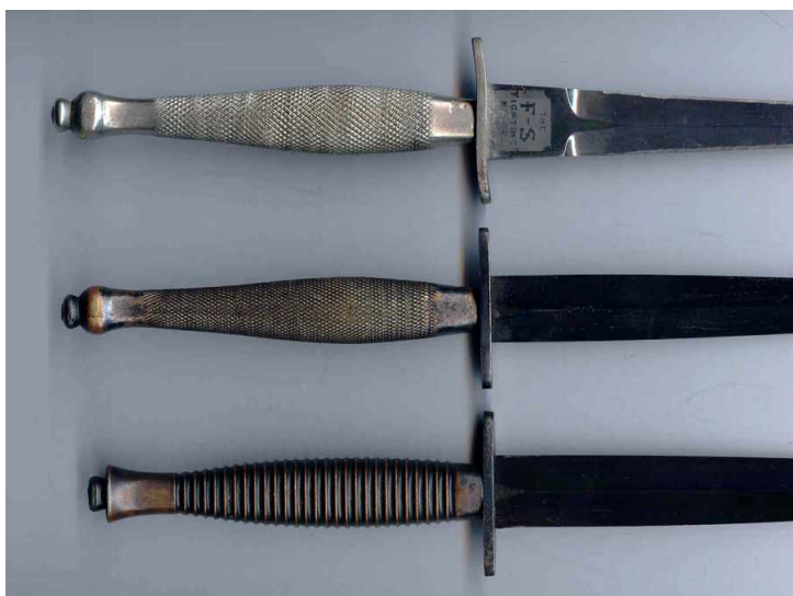
F-S knives: Top, 1st Pattern (from 11/1940), turned, knurled hilt, ricasso to blade with Wilkinson and FS markings, nickel plated. S-shaped early guards. Centre, 2nd Pattern (from 8/1941), no ricasso, blacked turned and knurled hilt, bright blade (blackened 1943). Bottom, 3rd Pattern (from 9/1942), blade as 2nd pattern, but with Rodgers' ringed alloy hilt. (Olof Jansen)
