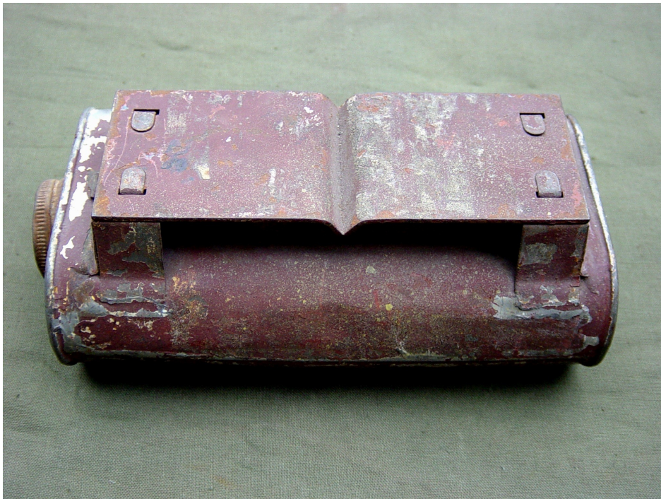
The 'Talcum Powder grenade', Hawkins grenade or No. 75 Mk I contained one and three-quarter pounds of Ammonal, Burrowite or Nobel's 704B. 200lb pressure on the top plate activated the crush igniters beneath. (Author's photograph)
