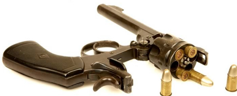
(Left) .455in Pistol, Revolver, No. 1 – formerly the Webley Mk VI service revolver – showing the weapon’s break action for reloading. (www.fmft.net)
