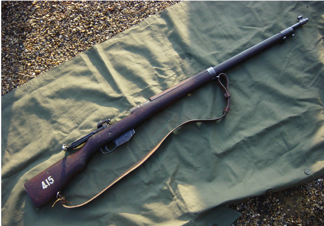
The lengthy Canadian .303in Ross rifle on the ranges at Bisley. This Mk 3 may well be one of the 75,000 purchased by the UK in 1940, as the only Ross adopted by the British Army was the Mk 3B, which was fitted with a magazine cut-off. (Author's photograph)
