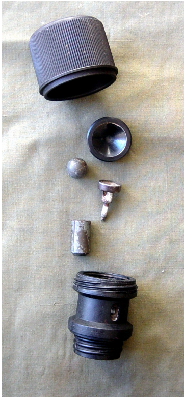
No. 247 'Bakelite' or 'All-ways' fuse dismantled. The safety cap (top) has been unscrewed from the fuse body (bottom), and the closing cap (second from top) removed, the concave underside of the closing cap is visible – which ensured that the fuse still operated if the grenade struck side-on. Below the closing cap is the ball, and below that the pronged striker (missing its creep spring), below the striker is the cap pellet. (Author's photograph)
