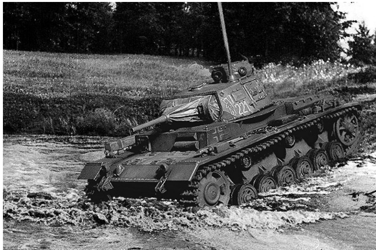
(Right): A PzKpfw III Tauchpanzer, showing the waterproofing on the gun mantlet and the snorkel erected. (www.mundosgm.com)
