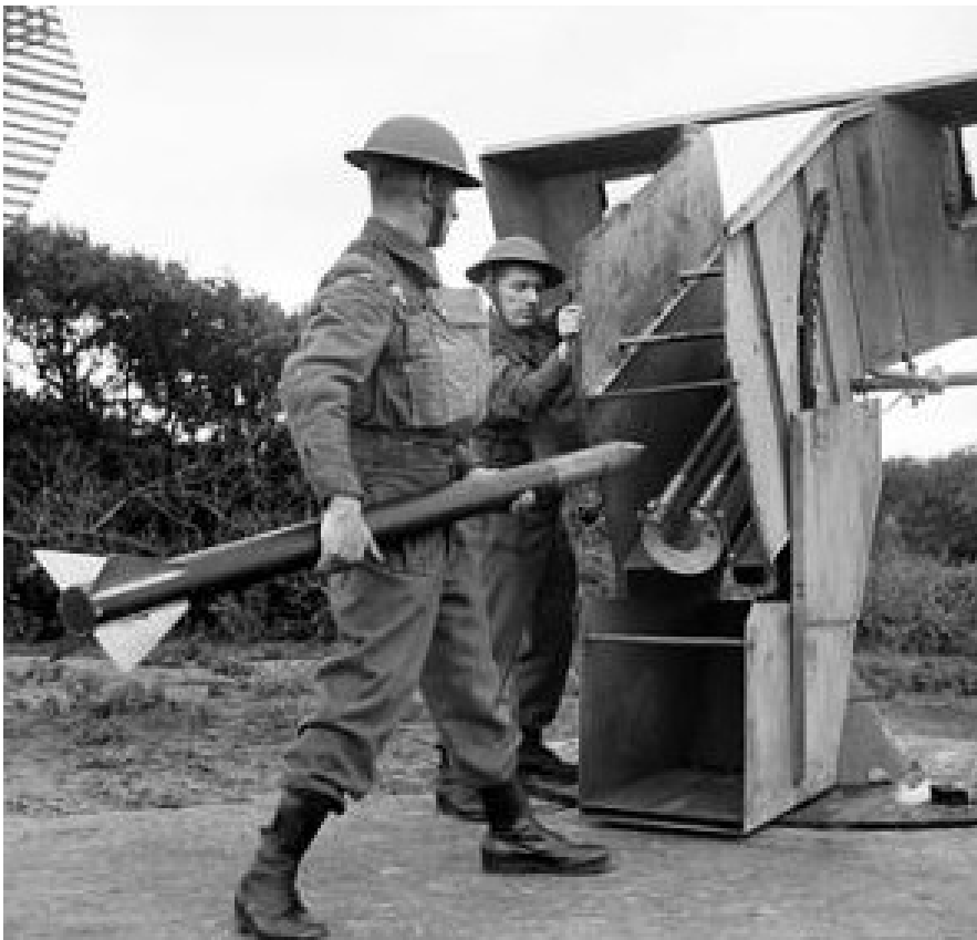
Home Guards on Merseyside loading a Mk I 'Z' projector, 6 July 1942. (IWM H 21135)
