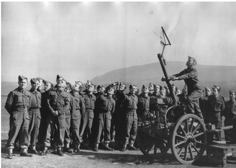
A Mk I (compressed air) Holman Projector demonstrated to a group of Royal Marines, July 1942. Note the anti-aircraft sight. A similar projector was emplaced to protect coastal defence guns at Tynemouth Castle. This example is mounted on a naval 12pr gun limber. Mk II projectors were steam powered; the Mk III was self-loading, but was not placed in production. (Official photograph, author's collection)
