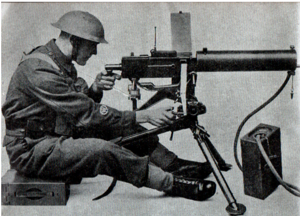
The M1917 Browning machine gun in British service, taken from the Gale and Polden booklet The Browning Heavy Machine Gun .300 calibre model 1919 (water cooled) Mechanism Made Easy, published in 1942. The firer is a Regular Army instructor, and the gun is mounted on the M1918 tripod. Note that the pistol grip is held with the left hand, while the right is used to adjust elevation and traverse. (Author's collection)
