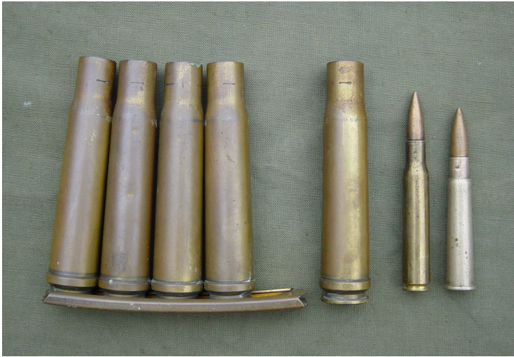
A charger of expended .55in Boys anti-tank rifle cases, with .30-06 and .303 bullets for comparison. These huge rifle rounds, were capable of defeating 21mm of armour at 300 yards. Although similar to the .50 Browning round, the Boys cartridge featured a belt around its base because of the very high pressures it developed. (Author's photograph)
