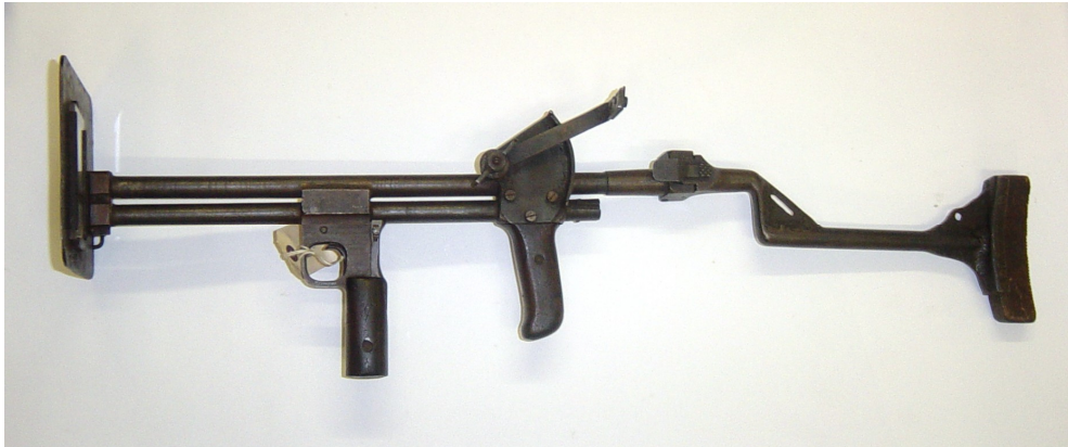
(Above) A folding-stock weapon that appears designed to fire a traditional stick tailed rocket from the upper tube, using a .22 cap firing mechanism in the lower tube. Note the elaborate sights, sling fittings, and blast shield.
