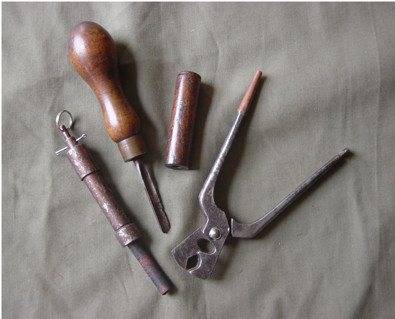
Explosives hardware – left to right, a pull switch for booby traps, an awl for making detonator holes in gelignite, awl blade cover with W^D marking, fuse cutter/crimping tool with copper clad prod for opening detonator holes. (Author's photograph)
