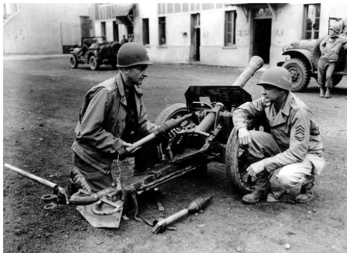
Right: US soldiers examine a captured ‘Püppchen’, in a view that clearly shows the conventional pressed steel carriage. A carriage like this would have greatly increased the utility of the 29mm Spigot Mortar and the 3in OSB Gun. (US Army official)
