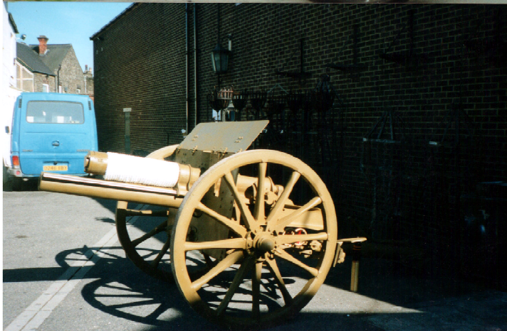
(Lower) Following cosmetic restoration by the author (in order to portray a QF 18pr in the recreation of the shelling of the Dublin General Post Office, in the feature film Michael Collins). The flat shield and shorter barrel (lacking the belled muzzle) differentiate this gun from the British 18pr. (Author's photographs)
