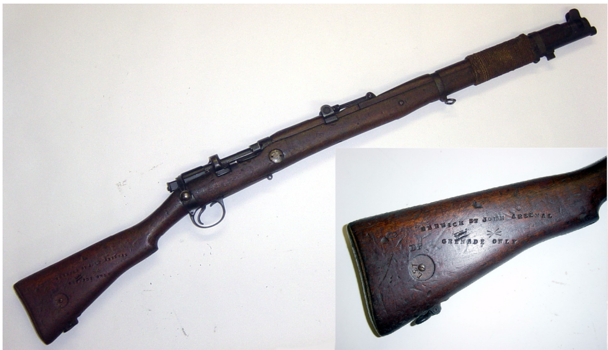
An EY rifle prepared by Mark Dinely's 'Berwick St. John Arsenal' for his Home Guard platoon (stamped on butt, inset). Note the lack of magazine, strengthening bolt below the breech and cord binding to the fore end. The stamps on the butt indicate that this particular rifle had been declared drill purpose only ('DP') and subsequently sold out of service (double broad arrow marks touching ><). Conversion to an EY rifle was making excellent use of an unserviceable weapon. (Author's photograph, reproduced by kind permission of Bapty & Co. Ltd.)
