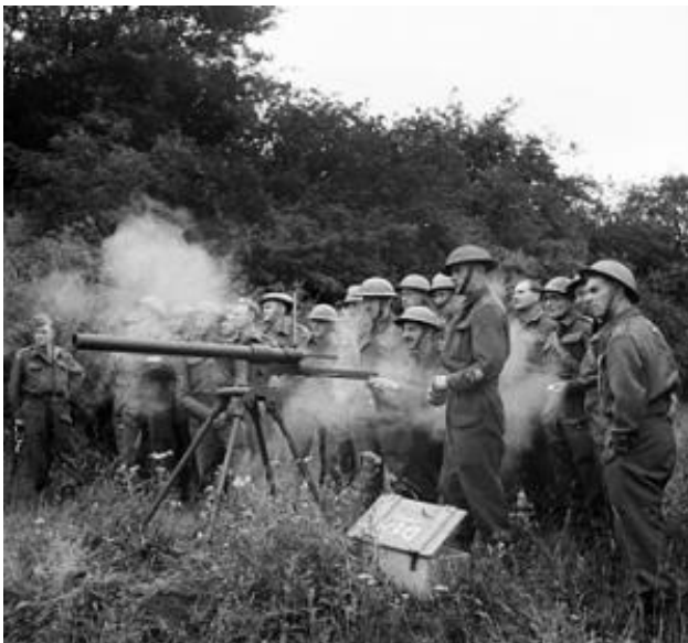
A War Office training team demonstrates a Mk I Northover Projector to members of Saxmundham Home Guard, 30 July 1941. The mount could be set much lower in operational use. The photograph illustrates the white smoke 'signature' generated by the Northover's gunpowder propelling charge. (IWM H12293)
