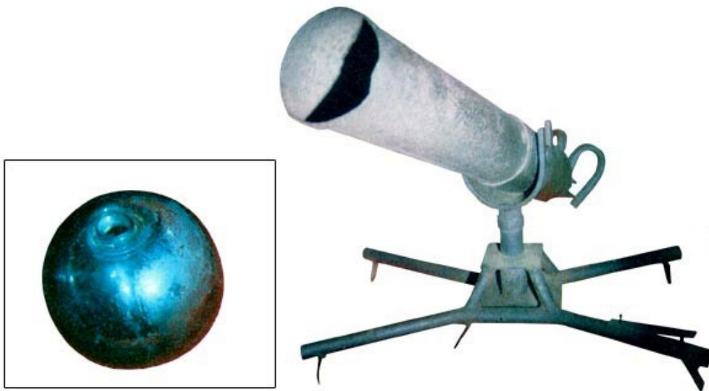
Soviet Ampulomet and its spherical glass projectile (inset). Compared to the Northover of 1940, this 'bottle mortar' of 1941 is decidedly unsophisticated. (www.sinopa.ee)
