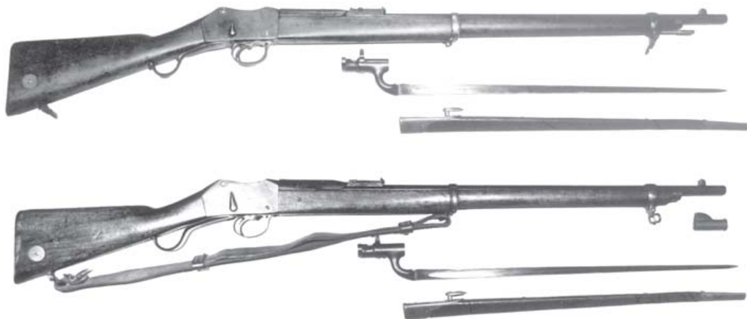
Martini-Enfield Rifles Mark I (above) and Mark II (below), each with Pattern 1895 Socket Bayonet and scabbard; the Mark II is accompanied by a protective nose cap. (Courtesy of Ian Skennerton)
