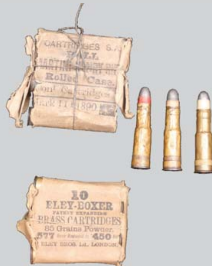
Cartridge packs and three .450in cartridges. The 480-grain round-nose bullet can be seen clearly. From left to right: blank cartridge, carbine cartridge and standard rifle cartridge. (Author)
