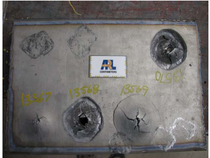
Figure 28. Production Acceptance Testing on a 4.00" Class 3 MIL-DTL-46077G Plate
