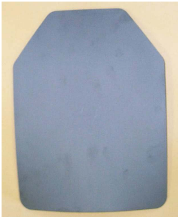
Figure 18. Hot-Pressed Net Shape Titanium Body Armor Plate
