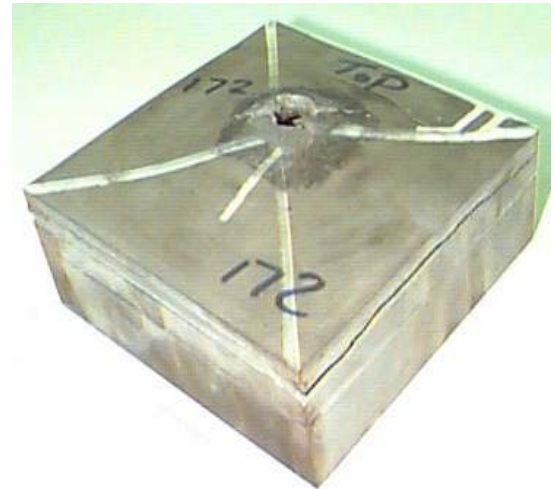
Figure 24. Hot Isostatically Pressed Ceramic in Titanium Matrices
