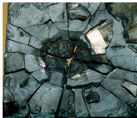
Figure 22 Functionally Graded Titanium Monoboride/Titanium Plate
