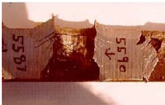
Figure 21. Hot Isostatically Pressed Ti-6Al-4V/CP Titanium Dual Hard Laminate
