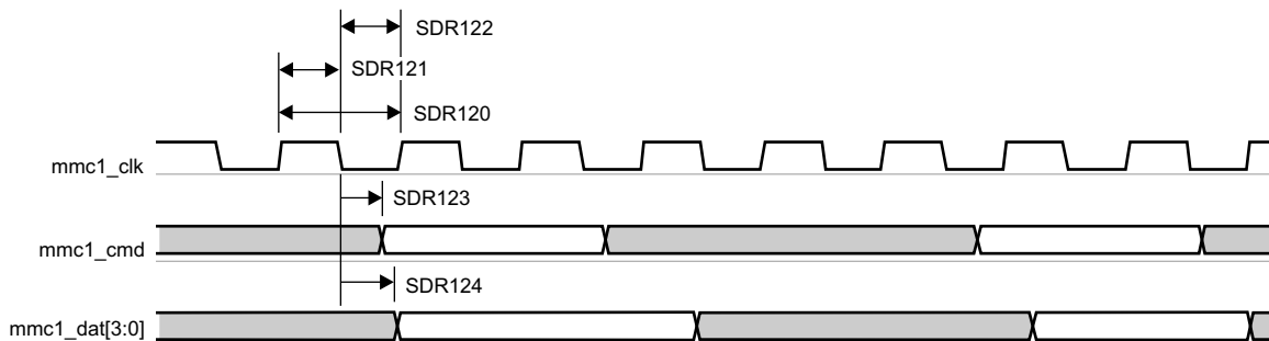
Figure 7-65. MMC/SD/SDIO in - High Speed SDR12 - Transmitter Mode
