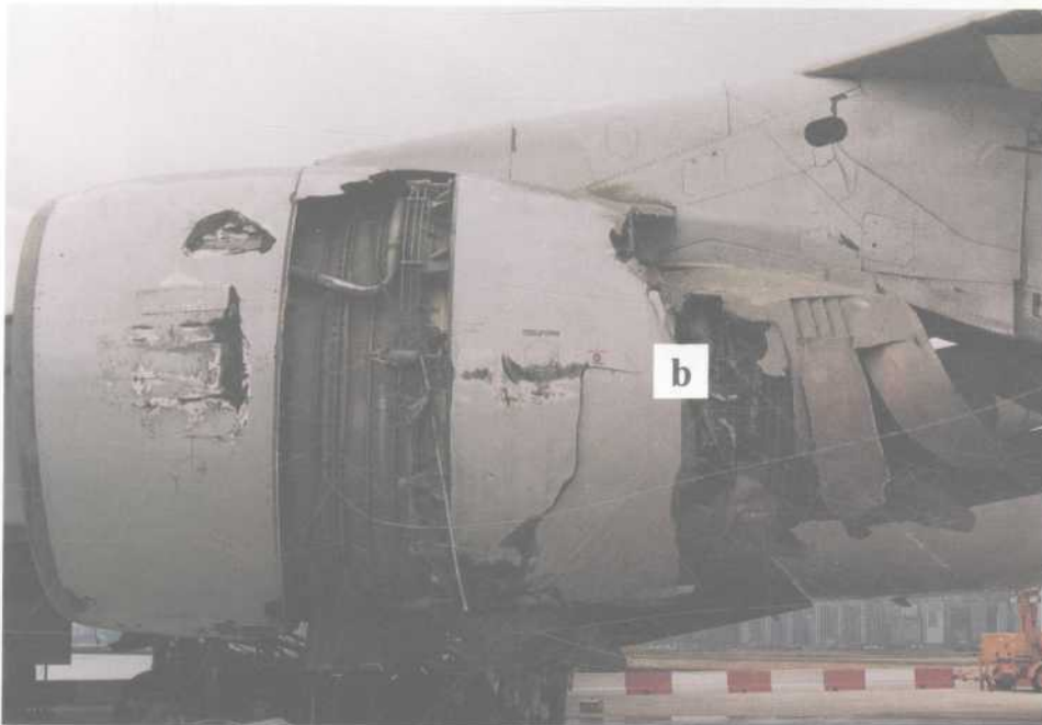
Damage to engine No 1 from sea wall strike along line 'a'. Secondary damage from prolonged contact with approach light structure marked 'b' Figure D
