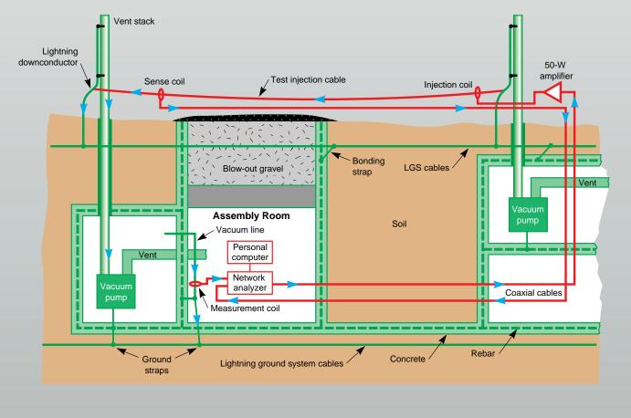
connect the vent stacks to the DAF's steel rebar and the facility's lightning grounding system.
