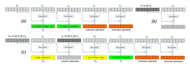
Figure 5: Detailed description of the attack on S/MIME. The original ciphertext is shown in (a). (b) is the canonical CBC gadget resulting in an all zero plaintext block. (c) is the modified ciphertext that is sent to the victim.
