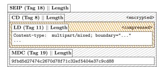
Figure 6: Nesting of a Symmetrically Encrypted and Integrity Protected Data Packet in OpenPGP. aged [30], and the two bytes are ignored. They depict the beginning of the first real plaintext block and the SE and SEIP packet types treat them differently.
