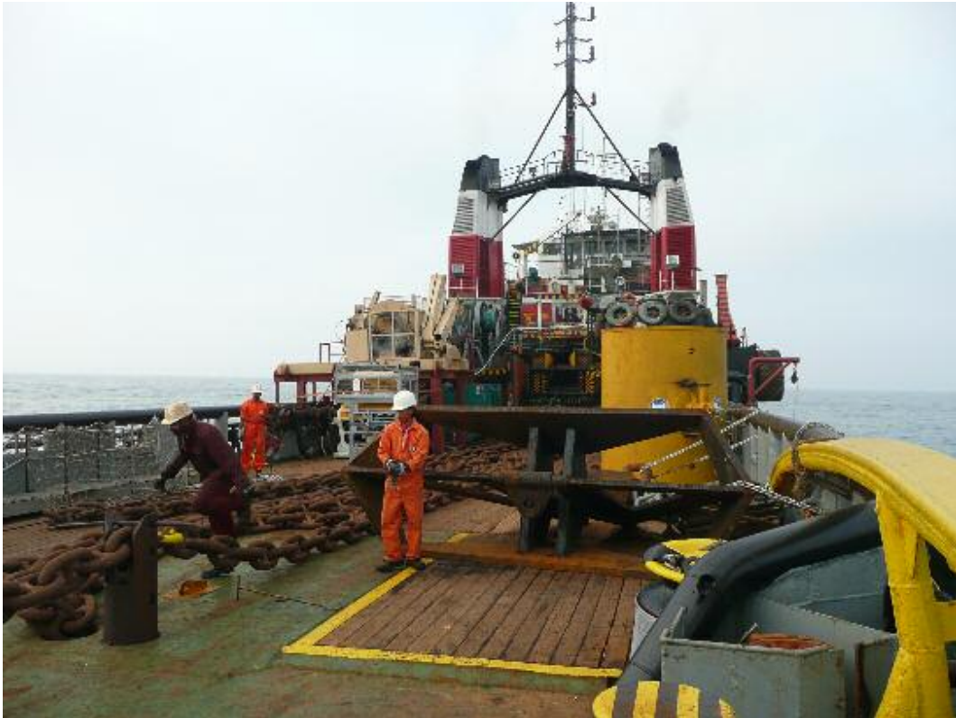
The Sri Lankan flagged AHT MAHANUWARA (former Smit-Lloyd 114 ) seen deploying an 4-point anchor system in the Straits of Taiwan.
