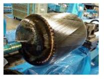
The filament wrap is bonded to the liner by a thin layer of adhesive. This adhesive is applied to the liner immediately prior to the filament wrap operation. After filament wrap, the vessel is placed in an oven and the resin is gelled and cured.
