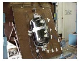
**Vibration Test, Sinusoidal and Random**: Qualification level sinusoidal and random vibration tests were performed on the Qualification Tank in each of the three principal axes. The vibration test requirements are shown in Tables 6 and 7.
