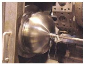
The outlet tube is made from 9.53 mm (0.375 inch) outside diameter tubing. The center section is fabricated from 0.5 mm (0.020 inch) thick CP-3 titanium sheet, rolled, formed, and welded into a cylinder with one longitudinal seam weld. This cylinder is manufactured using the same manufacturing technique as the previous helium pressurant tank center section.
