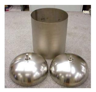
The pressurant tank liner was designed to mirror the construction of the previous pressurant tank liner. Although it has a slightly larger diameter, a forging was designed such that all four heads from these two tanks can be machined from the same forging configuration. The forging is made from CP 70 titanium bar. Figure 8 below shows a liner head being machined.
