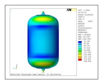
Figure 5a: Vibration Analysis, Lateral Random Stress Response of Liner
