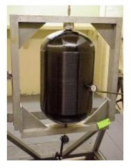
**External Leak Test**: The external leak test verifies the integrity of the tank shell and also serves to validate the previous series of pressure testing. The tank is placed in a vacuum chamber, which is evacuated to under 0.2 microns of mercury, and helium pressurized to MEOP for 30 minutes. The helium leak rate cannot exceed  $1 \times 10^{-6}$  std cc per second after a 30-minute stabilization period. For example, the leak rate of the Qualification Tank was 2.3 x  $10^{-8}$  scc/sec.
