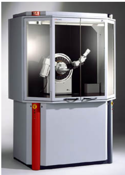
Figure 16: Bruker D8 Powder X-ray Diffractometer at X-ray Diffraction Laboratory [65], Department of Chemistry, Texas A&M University
