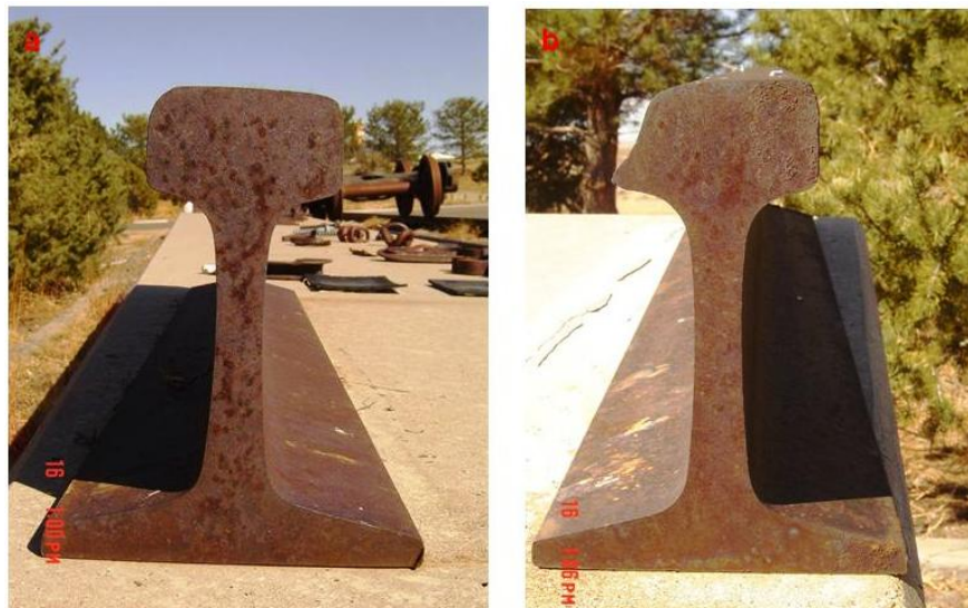
Figure 26: a) Undeformed rail b) Gage wear and plastic flow after service
