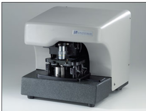
Figure 11: Nano-R™ Atomic Force Microscope (Pacific Nanotechnology Incorporated) at the Surface & Interface Science Lab, Texas A&M University
