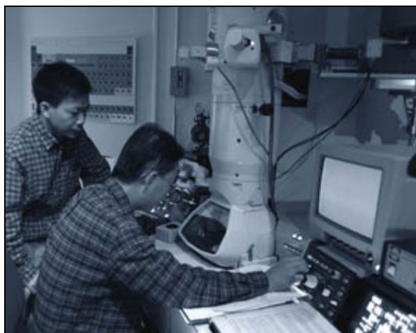
Figure 9: JEOL JEM 6400 Transmission Electron Microscope at Microscopy and Imaging Center [54], Texas A&M University
