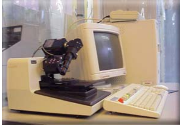
Figure 5: Dektet Profilometer at Materials Characterization Facility [39], Texas A&M University
