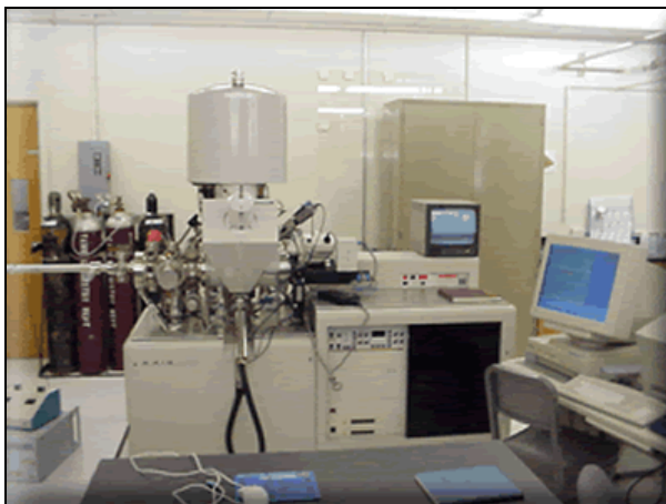
Figure 14: Kratos Imaging X-ray Photoelectron Spectrometer at Materials Characterization Facility [39], Texas A&M University
