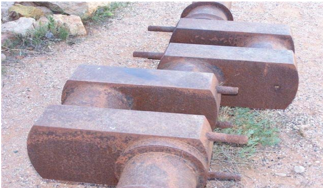
Plate 6. Crankshaft believed to be from one of the Wolf pumping engines originally installed at Umberumberka Pumping Station in 1915. The crankshaft is located in front of a shop in Silverton township a few kilometers from the pumping station. This may be all that remains of the original engines.
